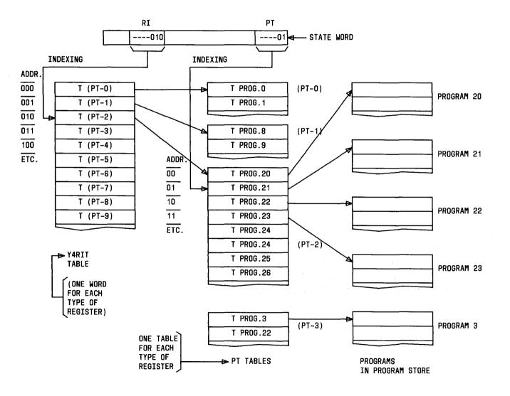
Fig. 4—RI-PT Method of Transferring to a Particular Call Processing Program
