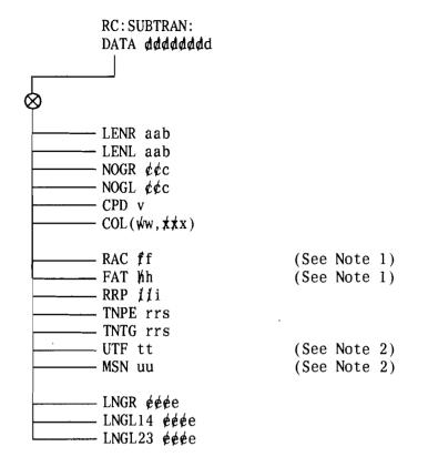
**Note 1:** For the RAC and FAT keywords, subtract octal 323 (decimal 211) from the block address to derive the actual subtranslator address to place into the head table. To seize a 1000-word block for a toll 3- or 6-digit translator or a 258-word block from an abbreviated 6-digit FAT, use key word LNGL14 (or LNGR if right half entries are desired).
