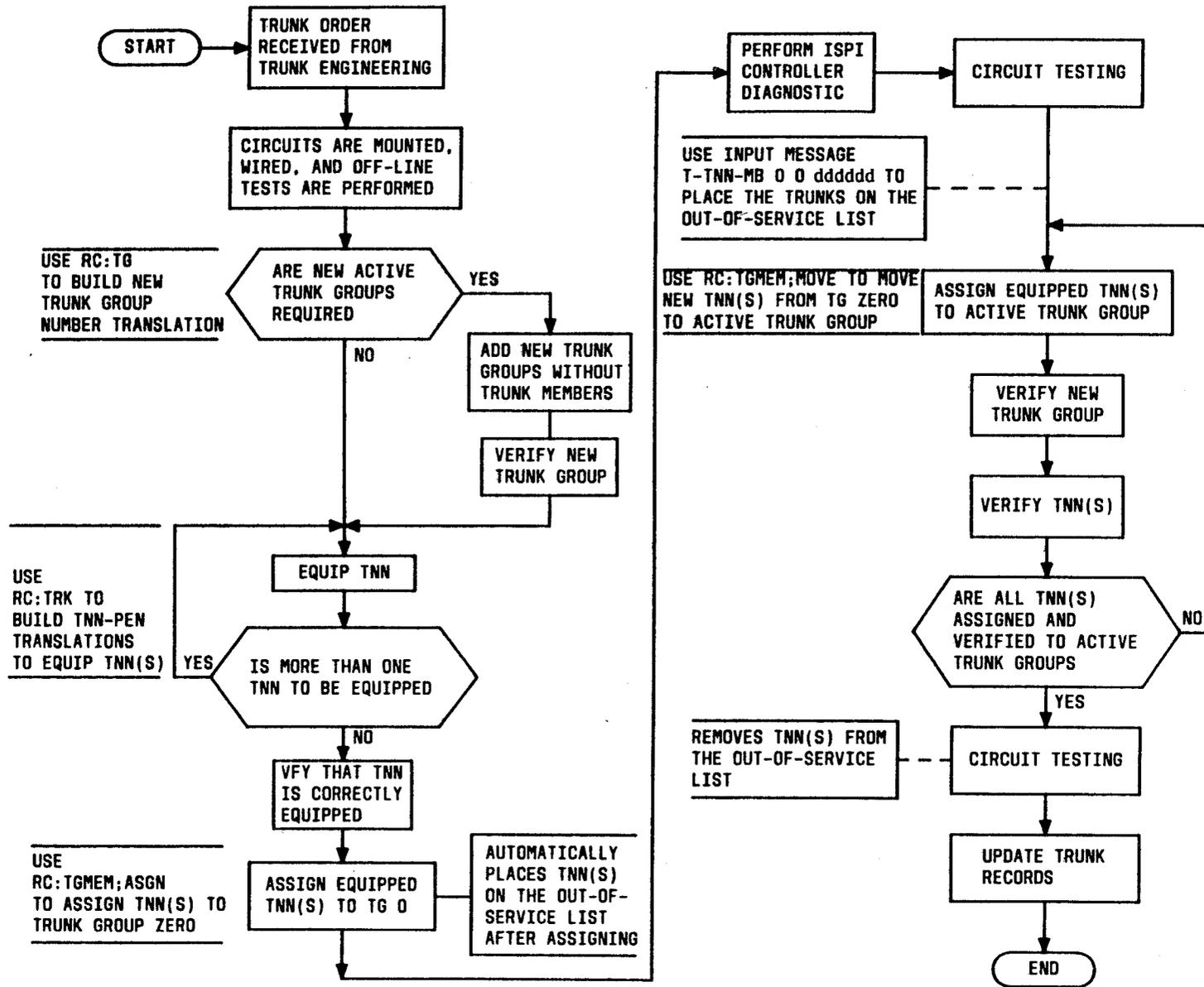
Fig. 11 — General Flowchart to Add a Trunk Circuit
