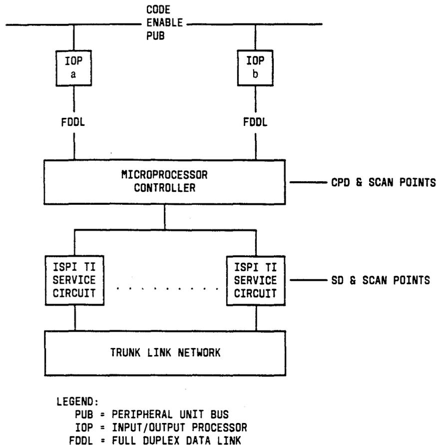
Fig. 1 — Typical ISPI Hardware Configuration
