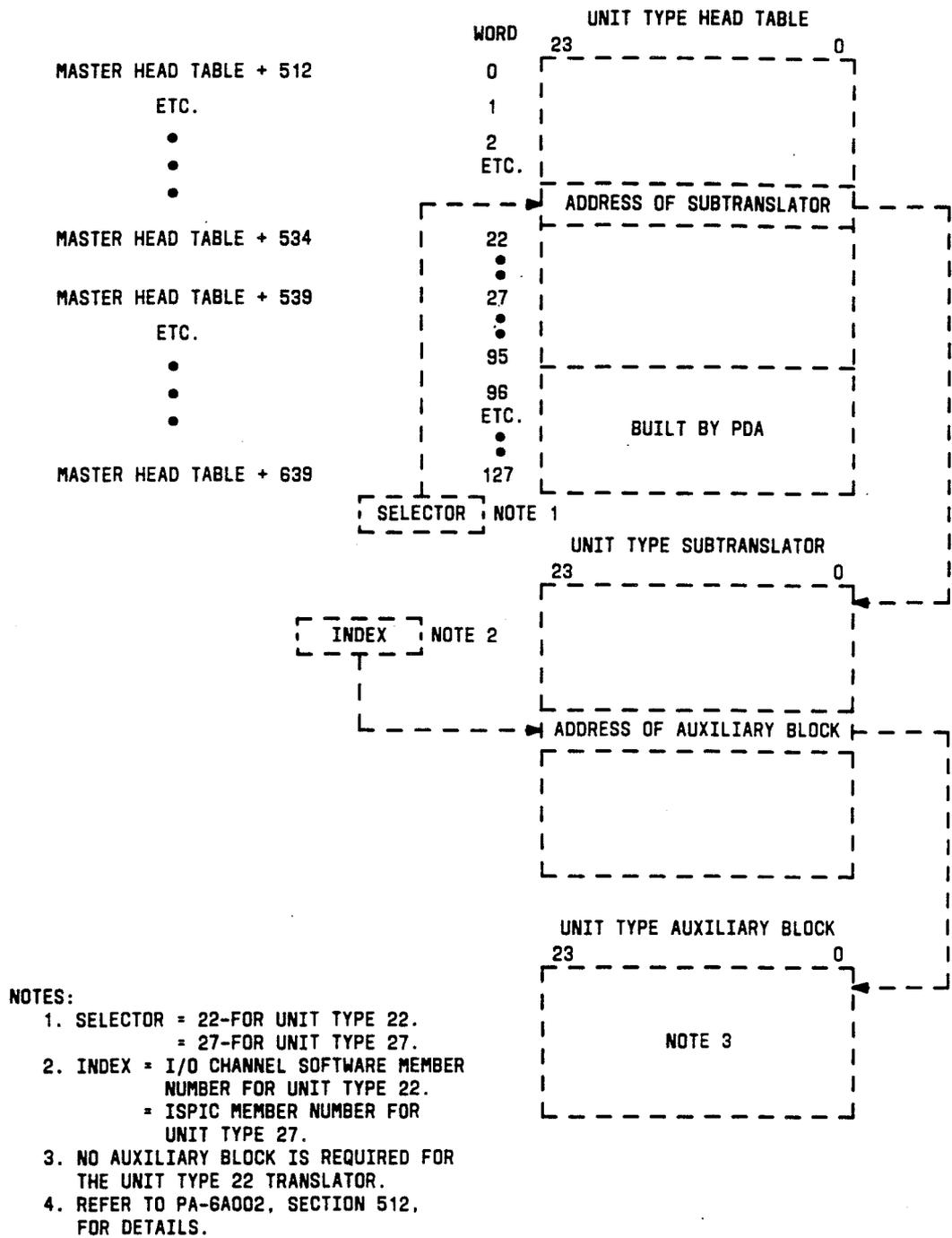
Fig. 6 — Flow Diagram for ISPI Unit Type Translators
