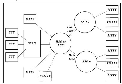
Figure 4-1: MTTY configuration in a DMS-10 cluster
