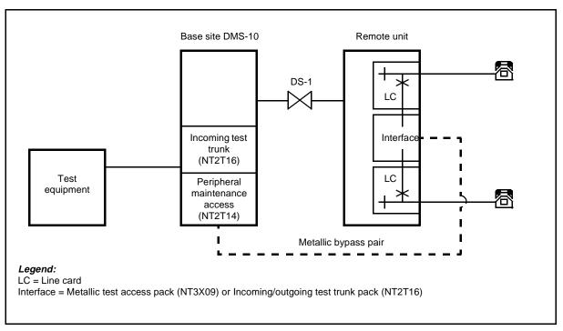
Figure 7-9: Metallic bypass pair test configuration for RLCM/OPM/OPAC
