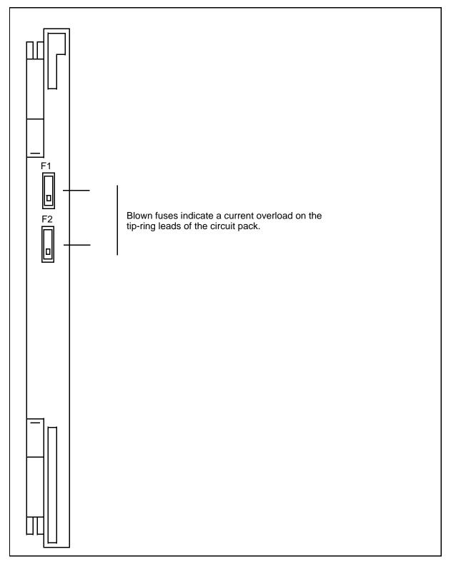
Figure 4-13: Line Test Unit-Analog pack faceplate (NT2X10)
