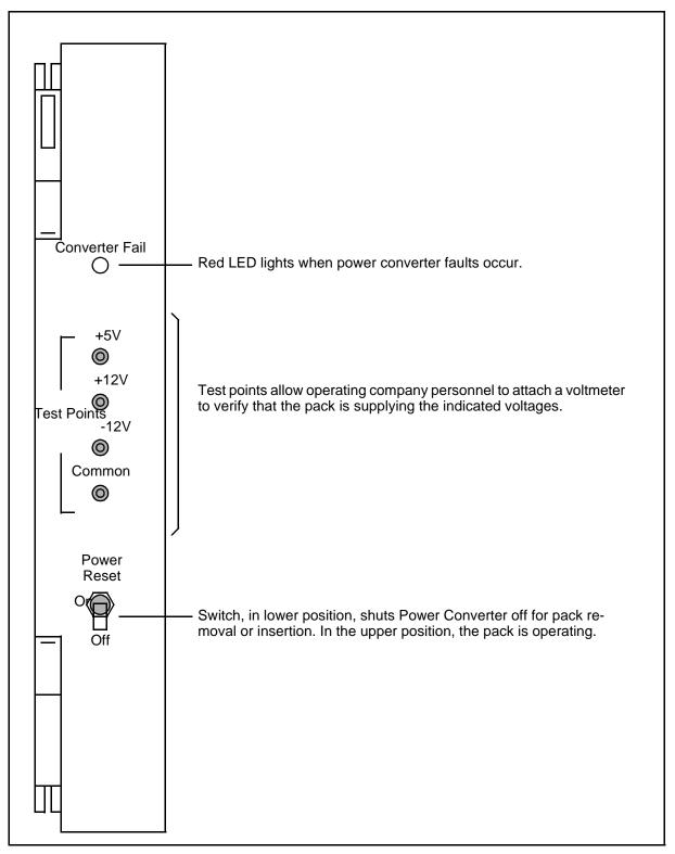
Figure 4-45: Power Converter pack faceplate (NTMX72)
