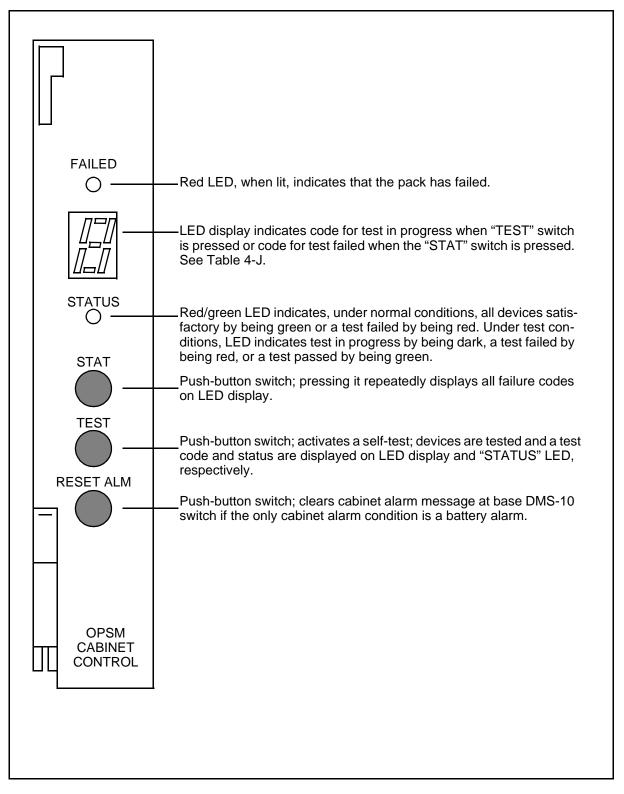
Figure 4-37: OPSM Cabinet Controller pack faceplate (NT9Y00)
