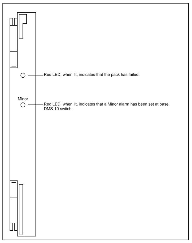
Figure 4-39: Remote Maintenance pack faceplate (NT9Y13)
