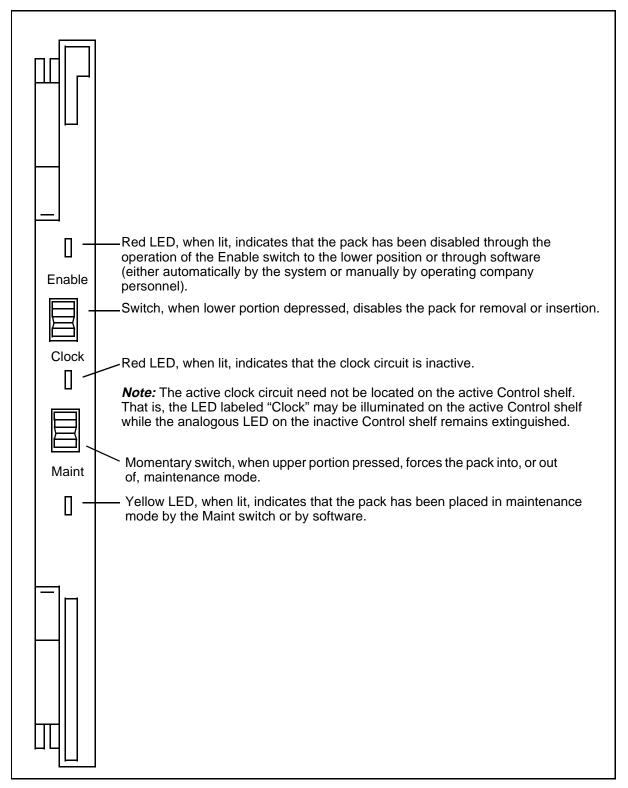
Figure 4-21: System Bus Controller pack (NT3T70BD) faceplate
