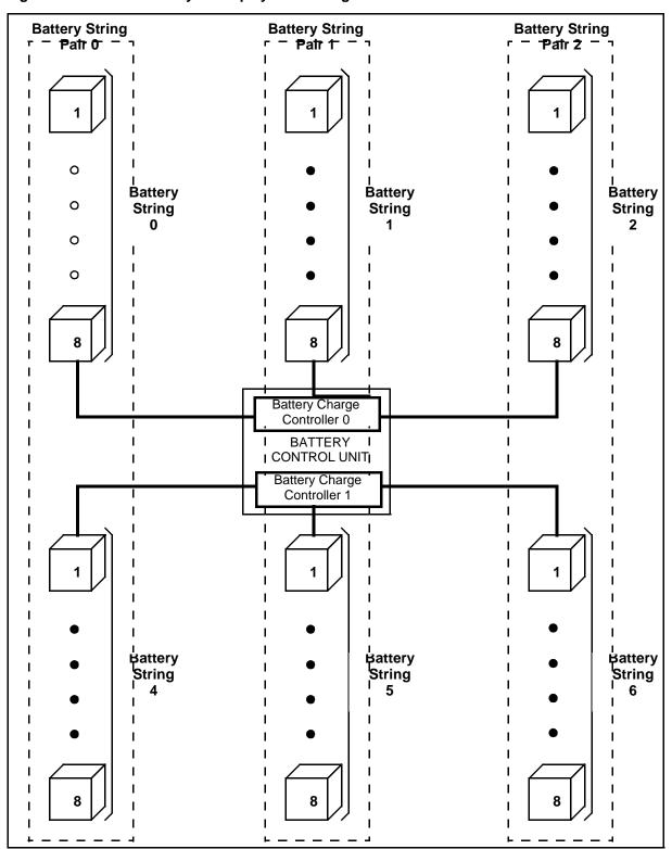
Figure 8-2: OPAC battery backup system configuration
