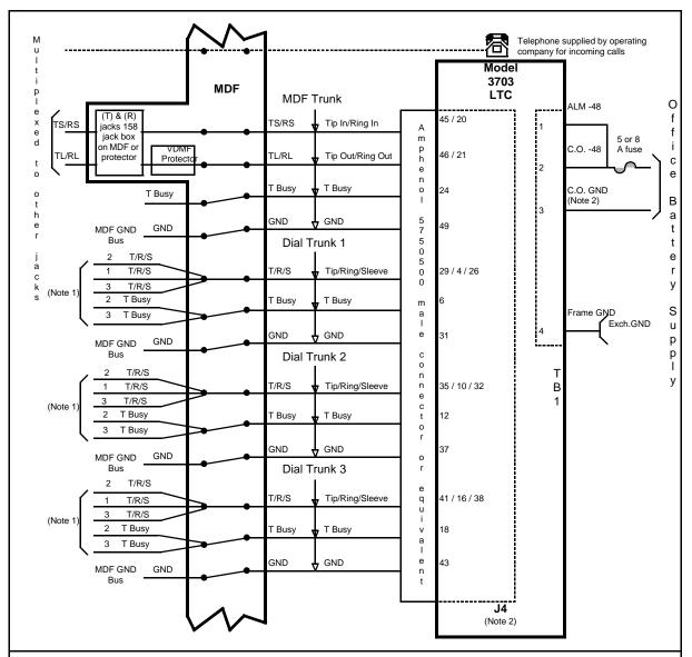
Figure 7-7: Connection between model 3703 local test cabinet and DMS-10
