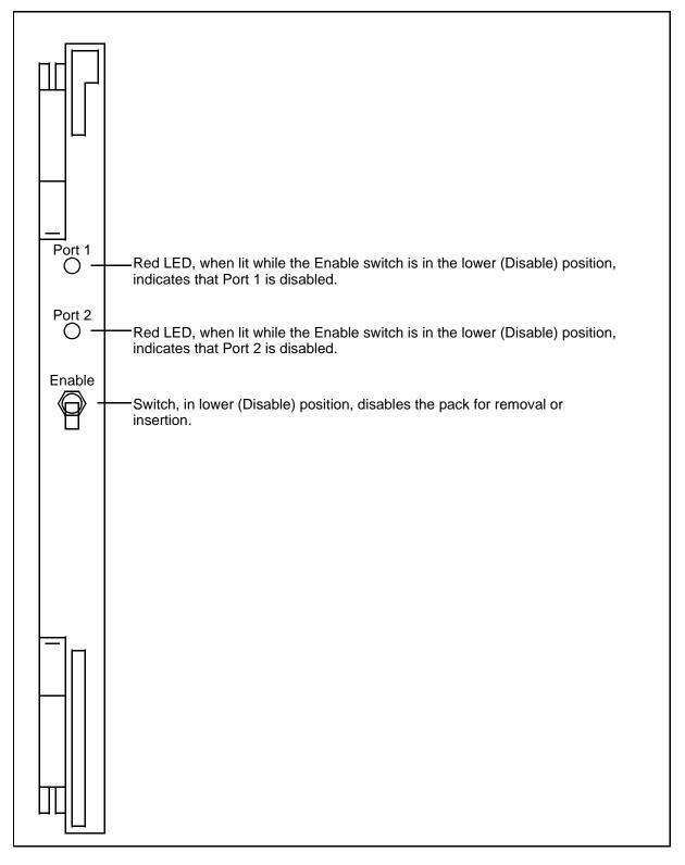
Figure 4-23: Dual Serial Data Interface pack faceplate (NT3T80BA)
