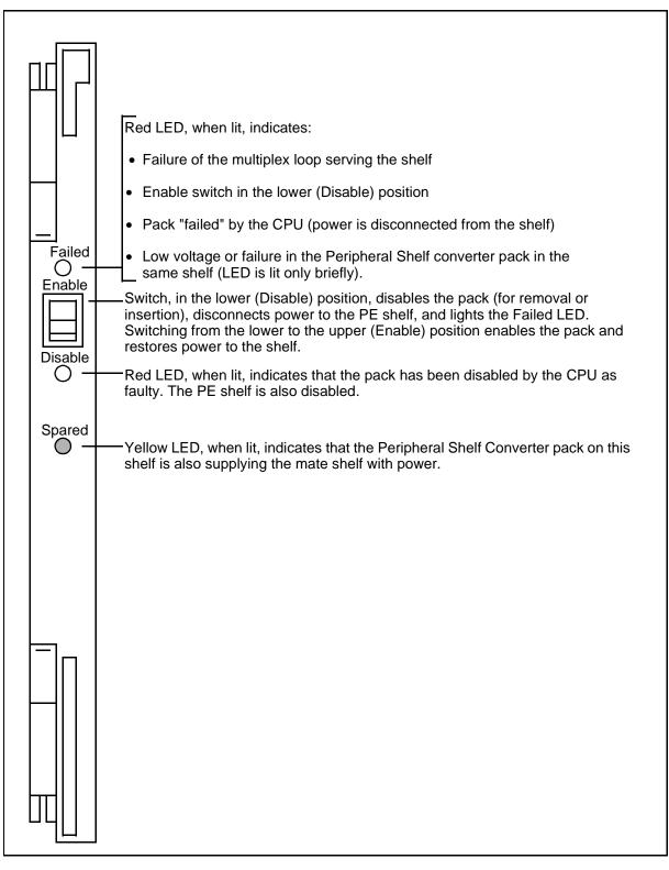
Figure 4-6: Peripheral Shelf Controller pack faceplate (NT2T41)
