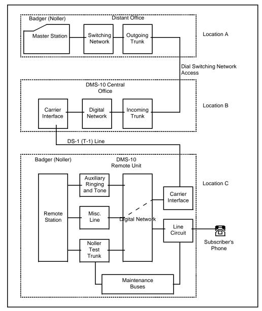
Figure 7-5: Badger to DMS-10 REM interface connections
