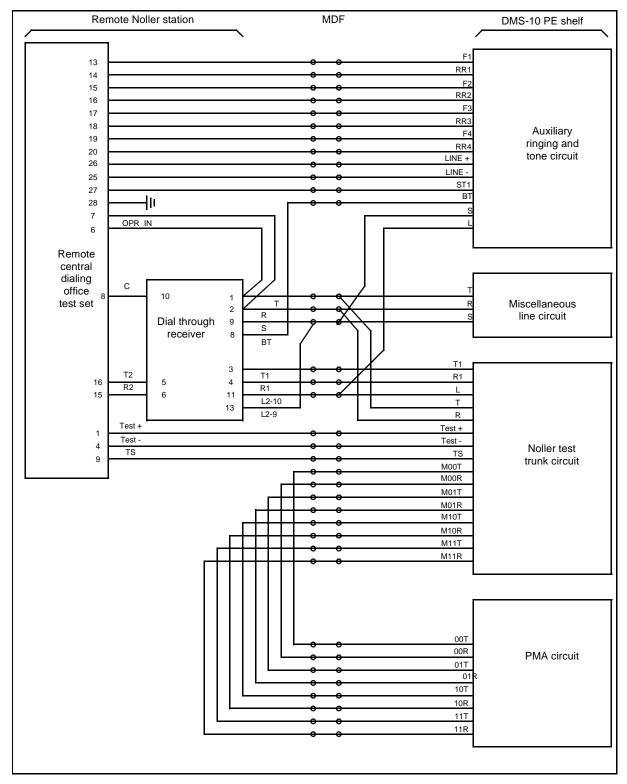
Figure 7-2: Noller to DMS-10 interface connections
