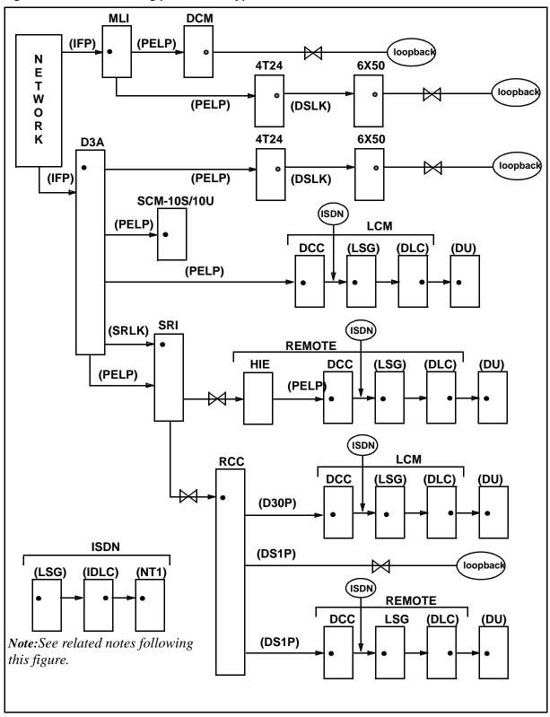
Figure 9-1: BERT testing paths - Path types
