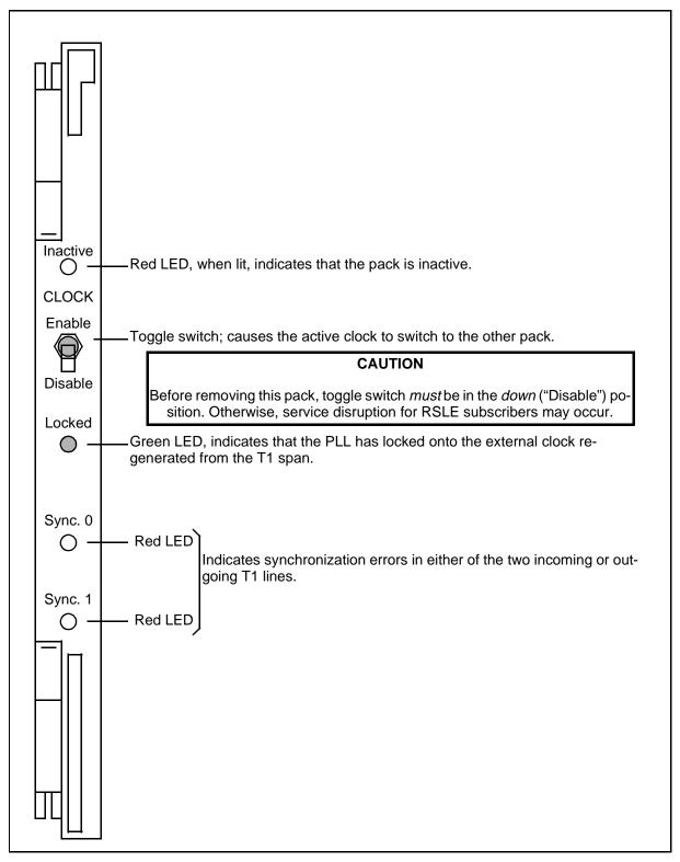
Figure 4-41: RSLE Dual Host Interface and Clock pack faceplate (NT9Y17)
