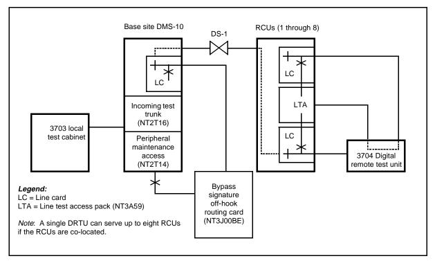
Figure 7-17: DRTU test configuration for RCU, SLC-96, and S/DMS AccessNode
