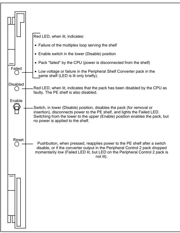
Figure 4-2: Peripheral Control 1 pack faceplate (NT2T12)
