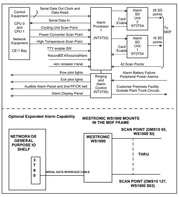
Figure 3-1: Alarm system with DMS-10 expanded alarm points block diagram
