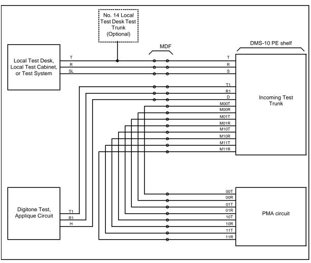
Figure 7-6: No. 14 LTD, no. 3 LTC, and CALRS connections
