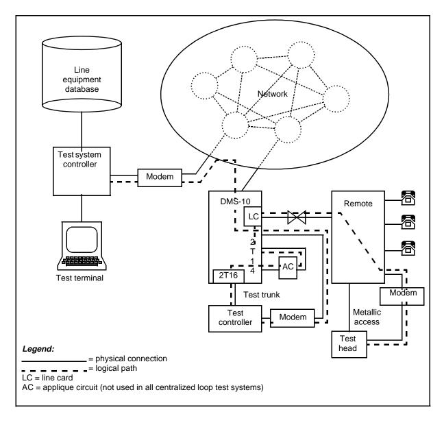
Figure 7-8: Typical DMS-10/remote centralized loop test configuration
