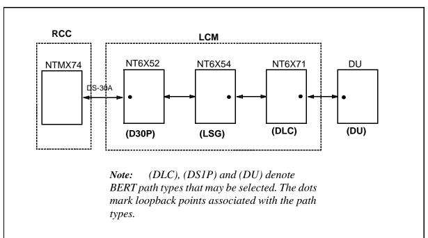
Figure 9-10: BERT testing paths - RCC to LCM
