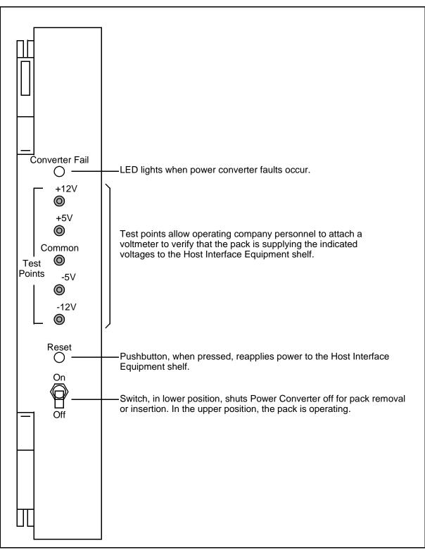
Figure 4-14: Power Converter pack faceplate (NT2X70)
