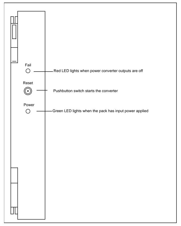
Figure 4-17: Power Converter pack faceplate (NT3T19AE and later)
