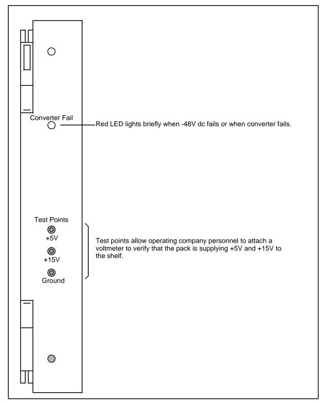
Figure 4-31: LCM Power Converter pack faceplate (NT6X53)
