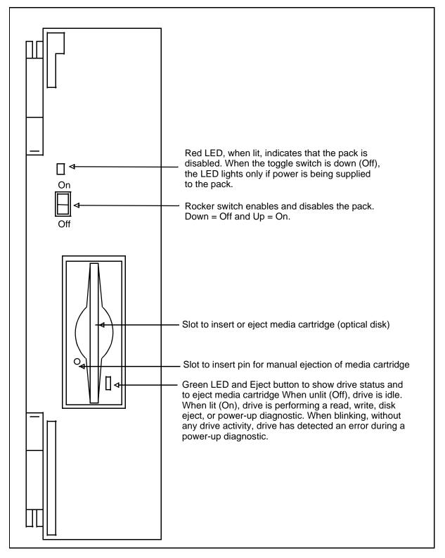
Figure 4-29: Magneto-Optical Mini-Disk Unit pack (NT4T32BA) faceplate
