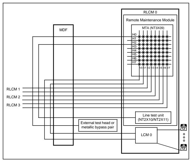
Figure 6-3: Metallic line access for Remote Line Concentrating Modules
