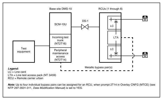
Figure 7-11: Metallic bypass pair test configuration for RCU
