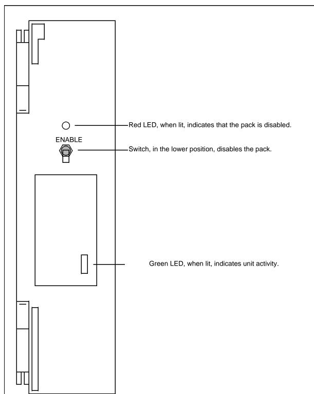
Figure 4-27: Hard Disk Drive faceplate (NT4T31AA)
