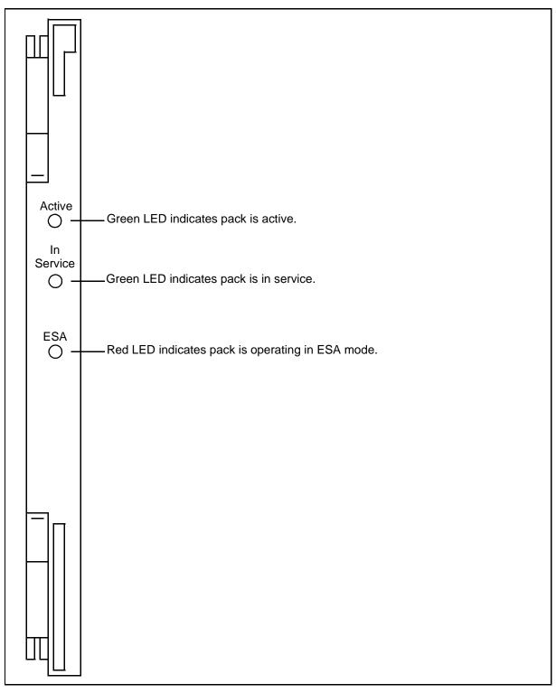
Figure 4-44: Cellular Application Processor pack faceplate (NTAX74)
