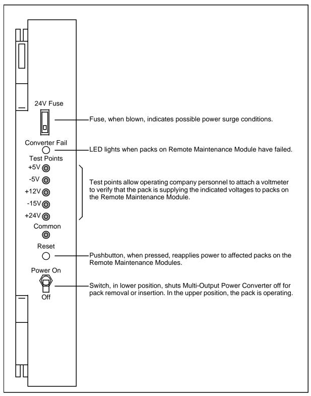
Figure 4-12: Multi-Output Power Converter pack faceplate (NT2X09)
