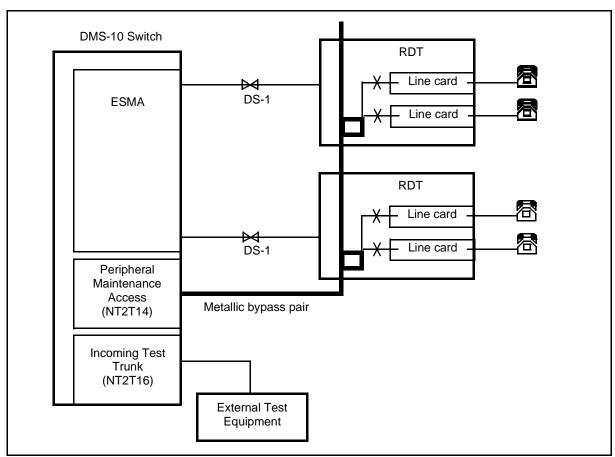
Figure 7-22: RDT line testing - metallic access from the host switch
