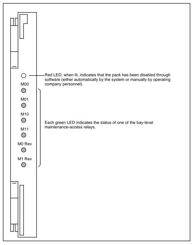
Figure 4-3: Peripheral Maintenance Access pack faceplate (NT2T14)
