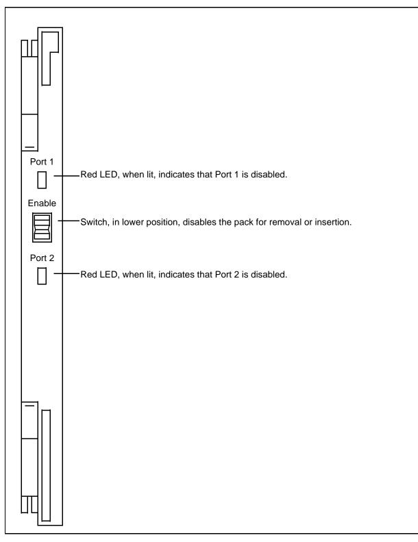
Figure 4-24: Dual Serial Data Interface pack faceplate (NT3T80BB)
