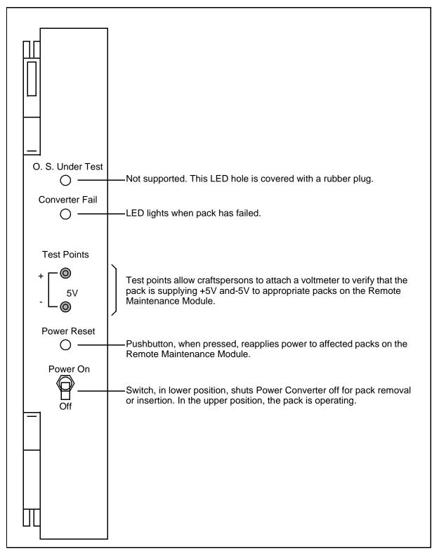
Figure 4-11: Common Feature Power Converter pack faceplate (NT2X06)
