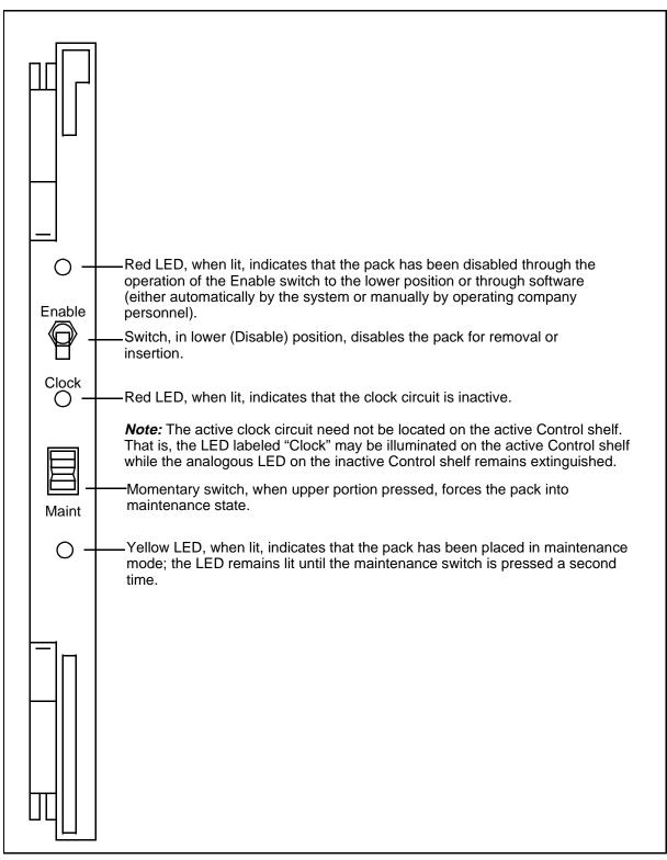
Figure 4-20: System Bus Controller pack faceplate (NT3T70BC)
