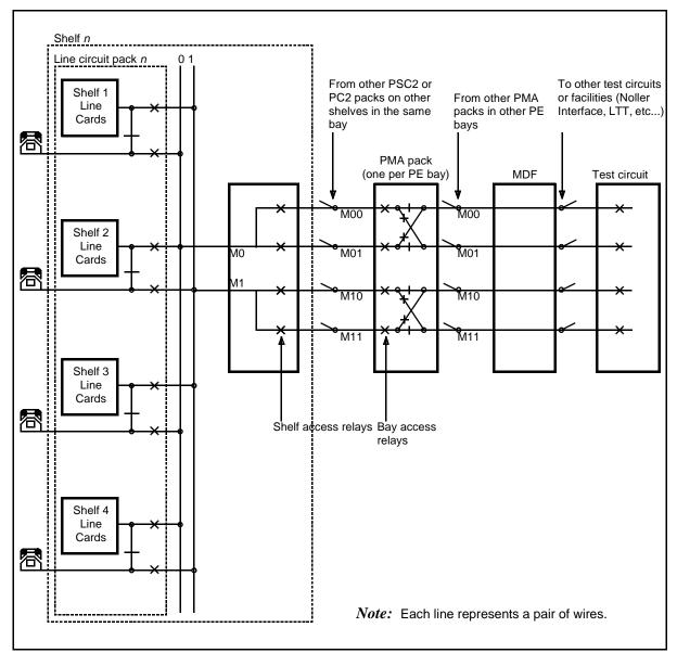
Figure 6-1: Maintenance bus for peripheral equipment
