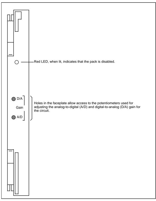
Figure 4-8: CAMA Position Signaling pack faceplate (NT2T48)
