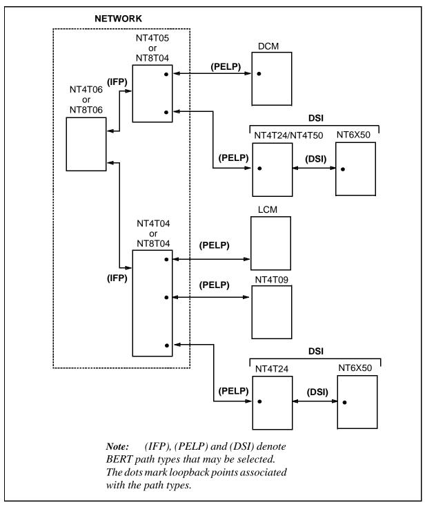
Figure 9-3: BERT testing paths - Network equipment
