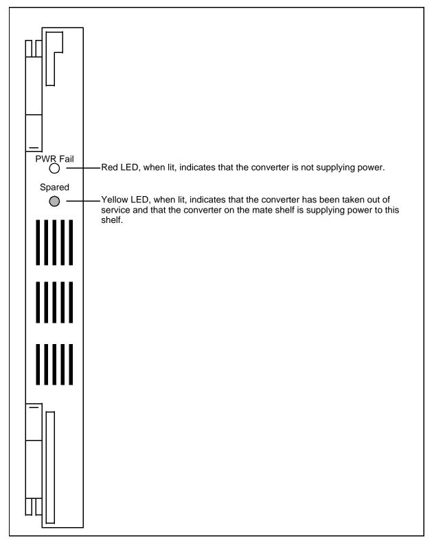
Figure 4-7: Peripheral Shelf Converter pack faceplate (NT2T42)
