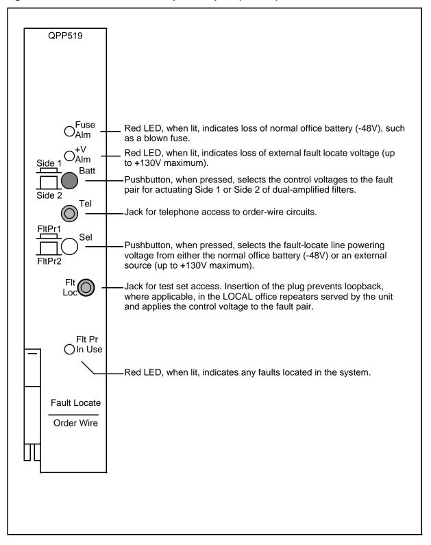
Figure 4-49: Fault Locate Order Wire pack faceplate (QPP519)
