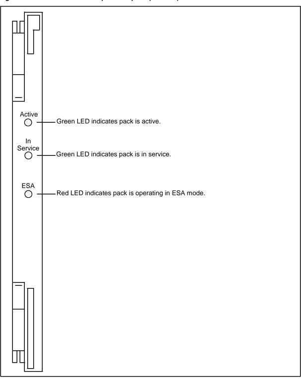
Figure 4-46: Unified Processor pack faceplate (NTMX77)
