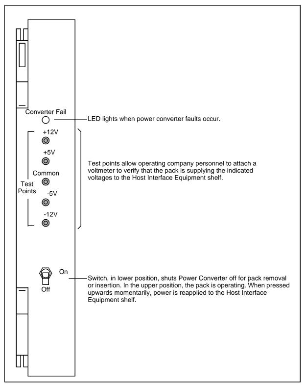
Figure 4-15: Power Converter pack faceplate (NT2X70AE)
