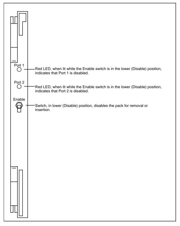
Figure 4-25: Dual Integrated Modem pack faceplate (NT3T93)
