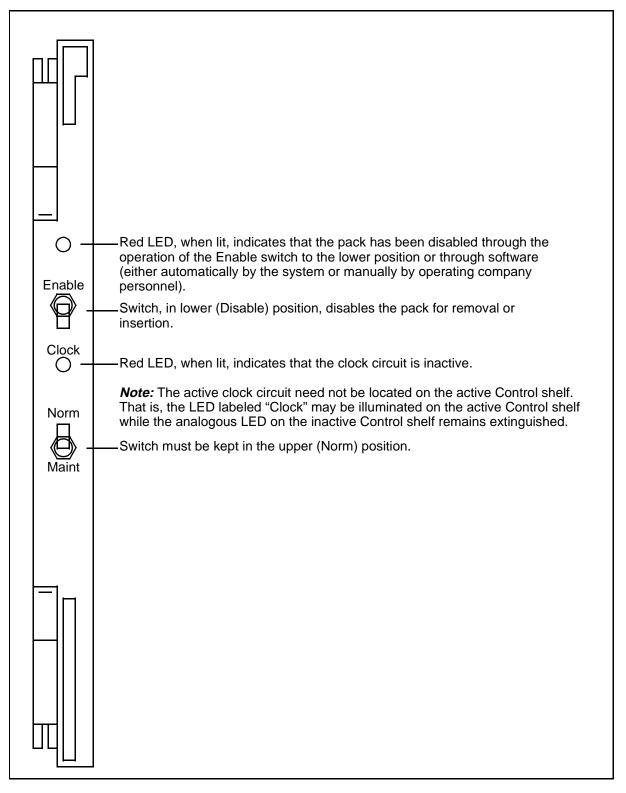
Figure 4-19: System Bus Controller pack faceplate (NT3T70BA)
