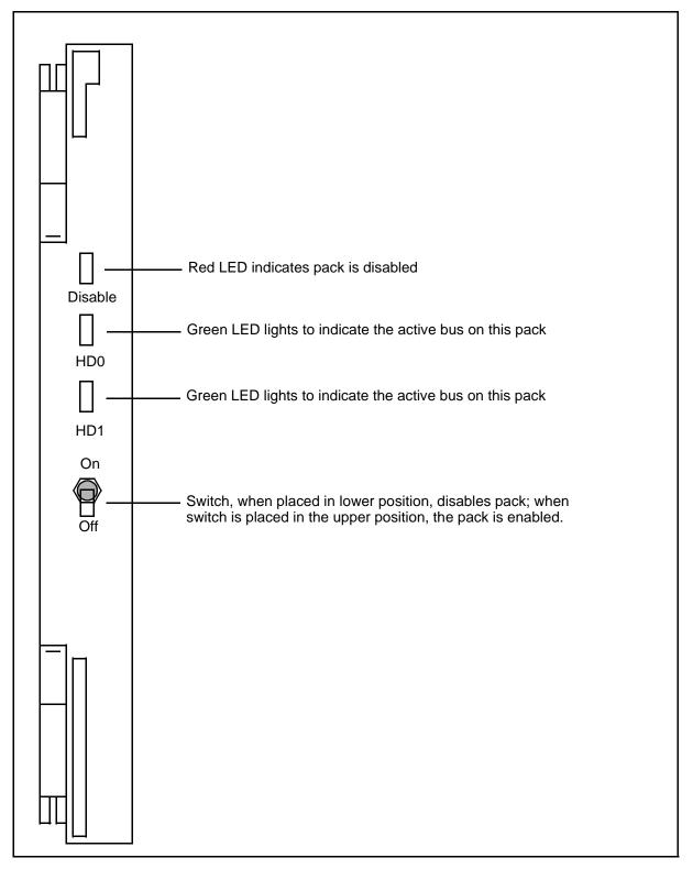
Figure 4-35: SCSI Bus I/O and Disk Drive pack faceplate (NT8T90)
