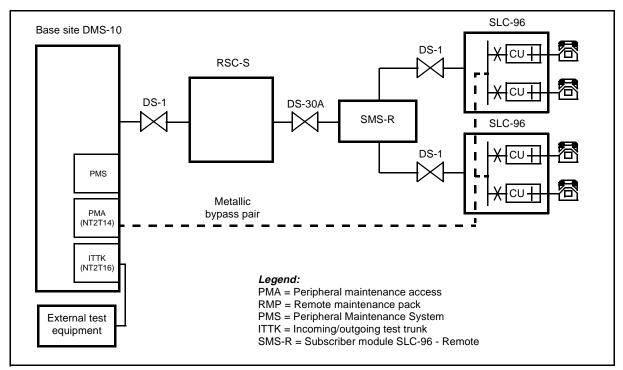
Figure 7-14: Test configuration for SLC-96 as RSC-S remote - Metallic access from DMS-10 host
