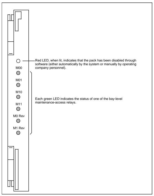
Figure 4-9: Facility Test pack faceplate (NT2T72)
