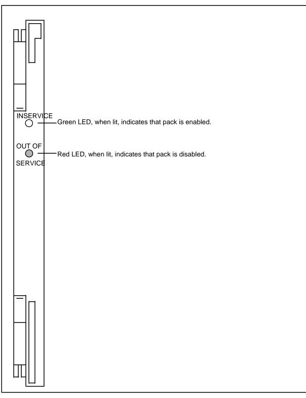
Figure 4-30: LCM Processor pack faceplate (NT6X51AC)
