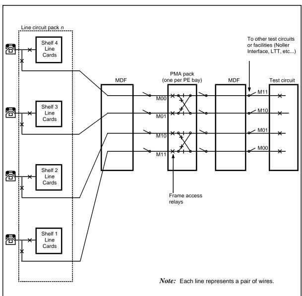
Figure 6-2: Maintenance bus for line concentrating equipment
