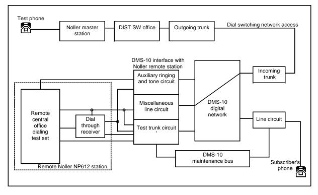
Figure 7-1: Interconnection between the DMS-10 switch and Noller NP612
