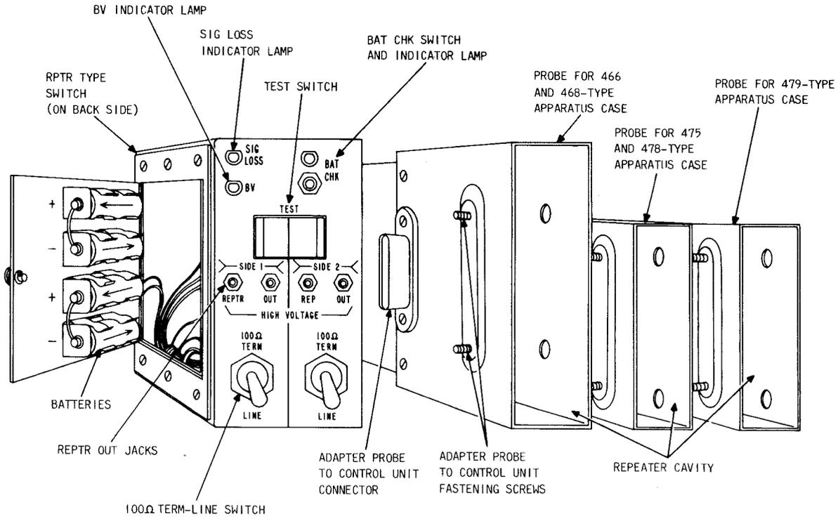
Fig. 7—J98725AB (25AB) Bipolar Violation Detector
