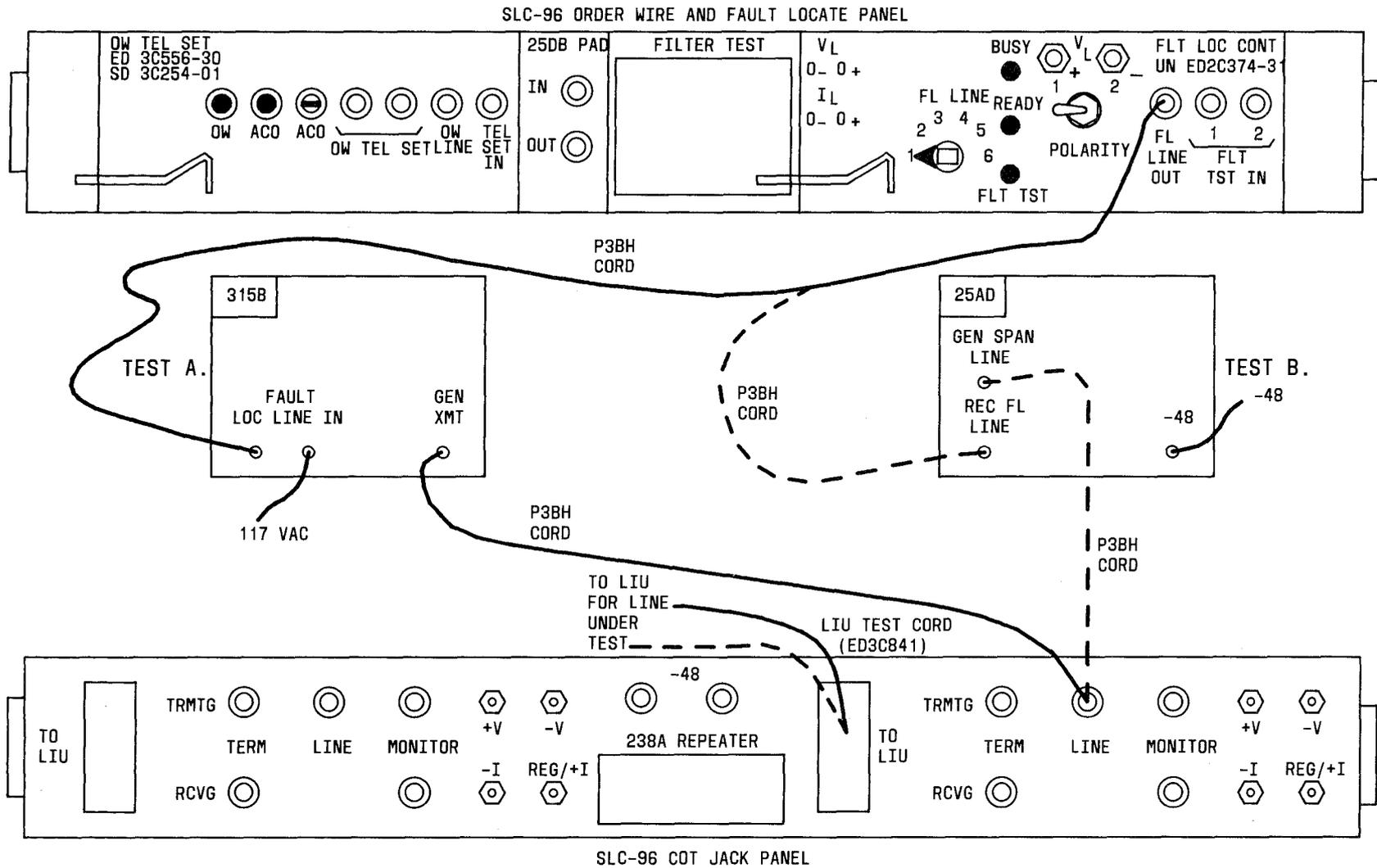
— TEST A. - TEST SETUP AT COT USING 315B TEST SET
