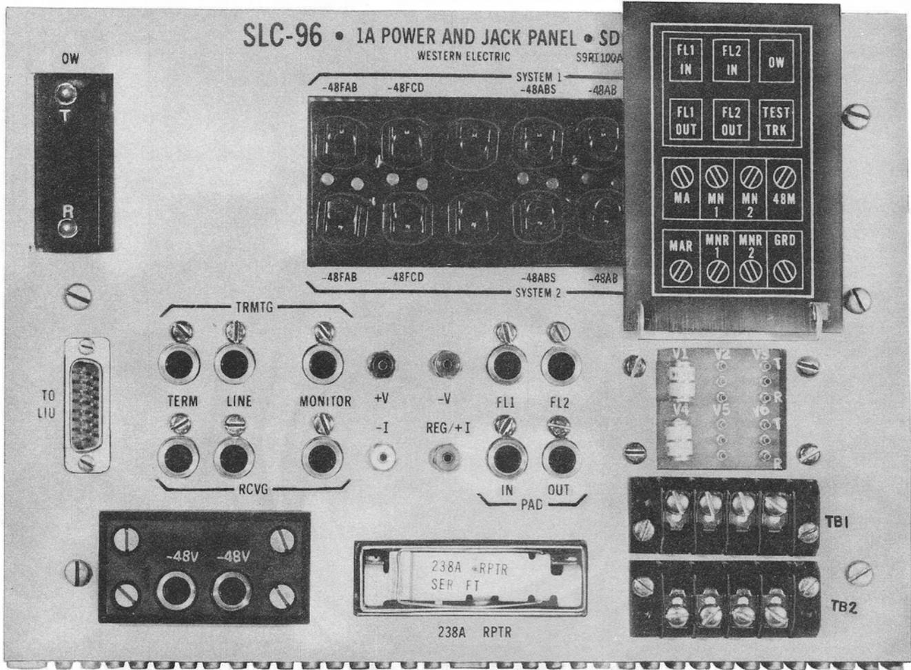
Fig. 9—SLC-96 RT 1A Power and Jack Panel
