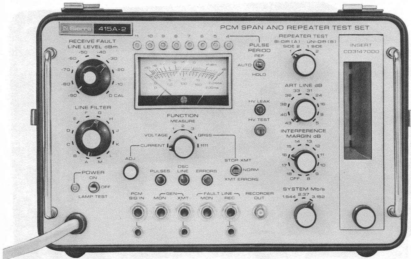
Fig. 3—Sierra 415A-2 PCM Span and Repeater Test Set
