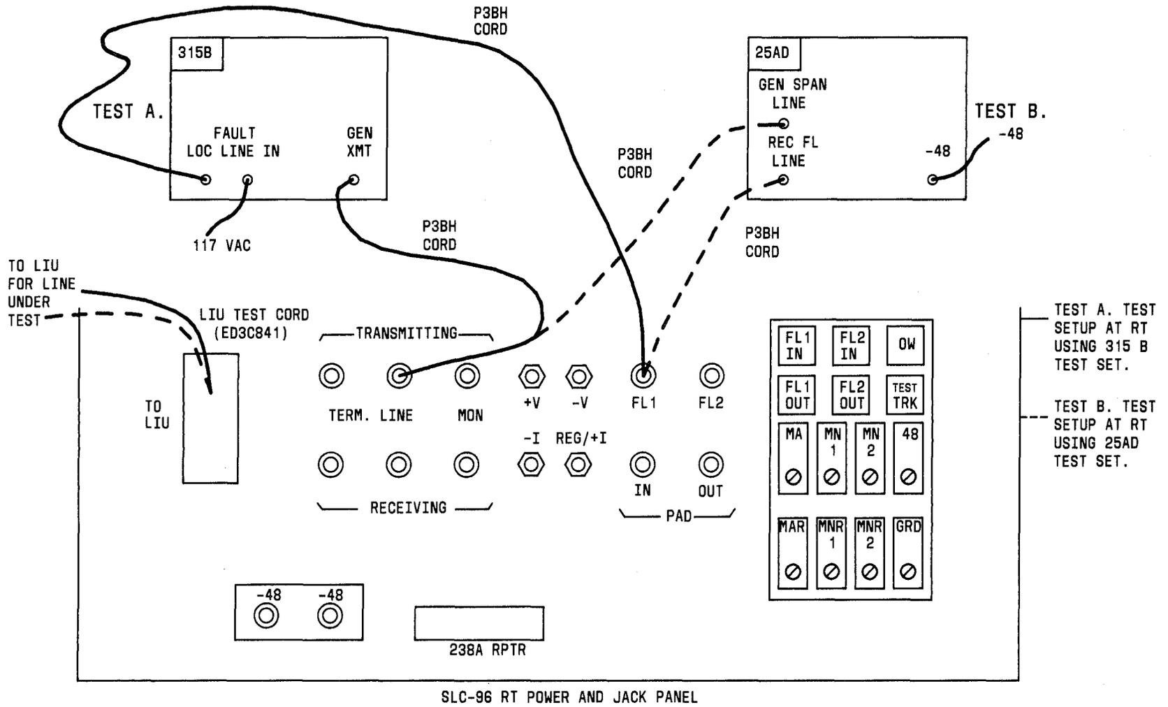
Fig. 18—RT Fault-Locating Configurations
