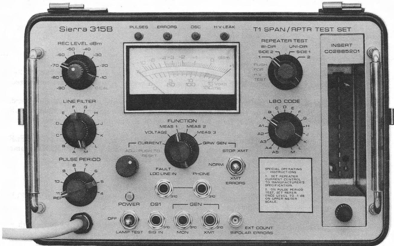
Fig. 2—Sierra 315B T1 Span and Repeater Test Set
