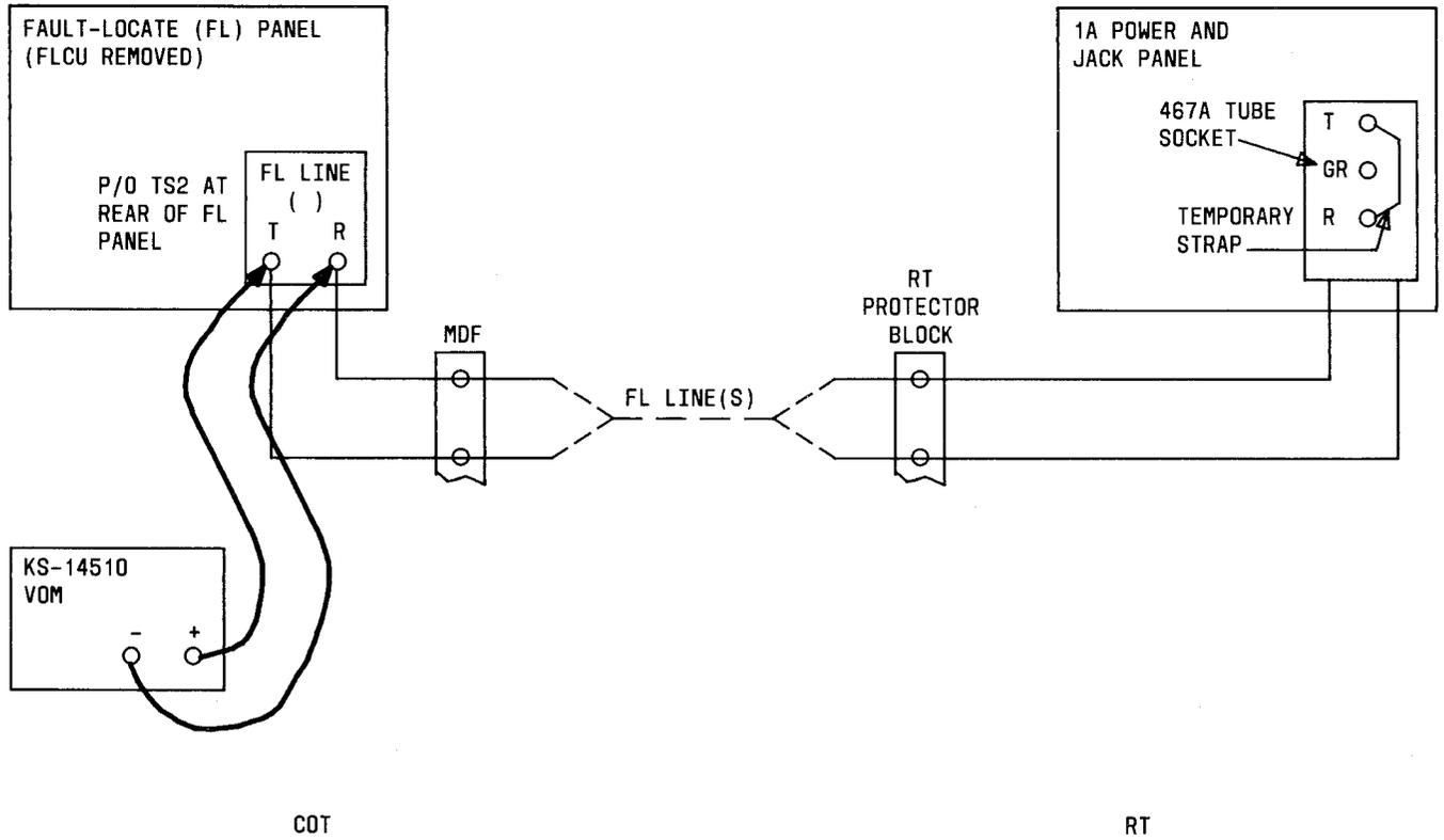
Fig. 10—DC Loop Resistance Test Setup
