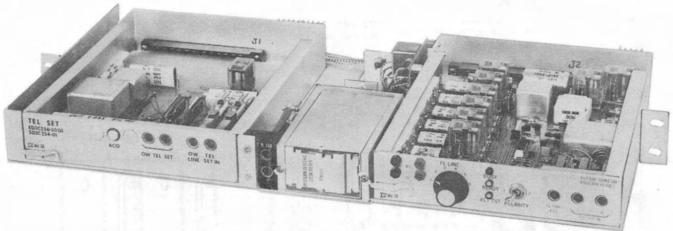
Fig. 5—COT Fault-Locate and Order Wire Panel (J1C141AC-L1)
