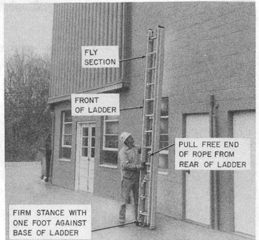
Fig. 23—Preparing to Extend Fly Section
