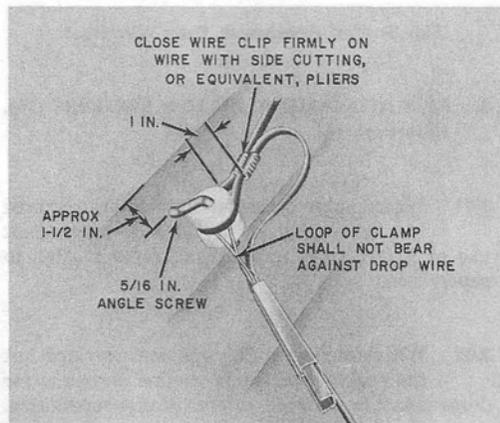
Fig. 1—First Attachment, Horizontal Run
