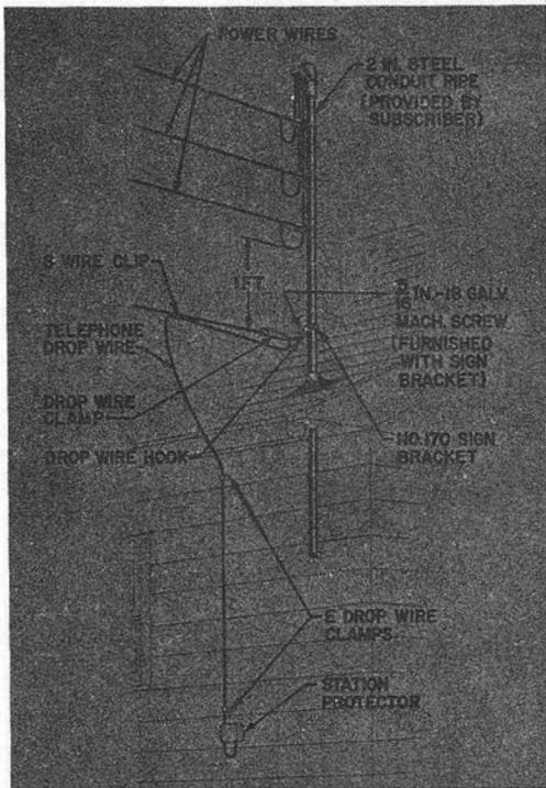
Fig. 10—Drop Wire Attached to Power Fixture
