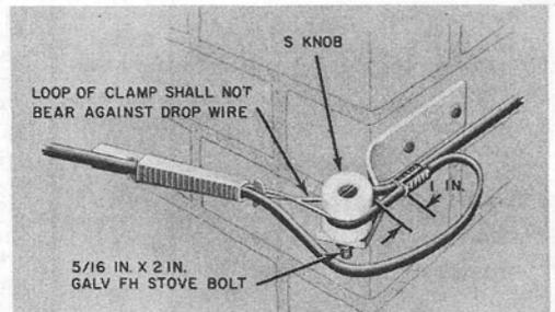
Fig. 8—First Attachment, Corner Bracket Using S Knob
