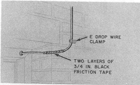
**Fig. 19—Last Attachment, Building Entrance Slopes Upward From Outside**
