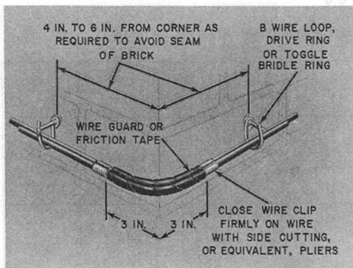
**Fig. 14—Spacing Attachments at Outside Corner of Building**
