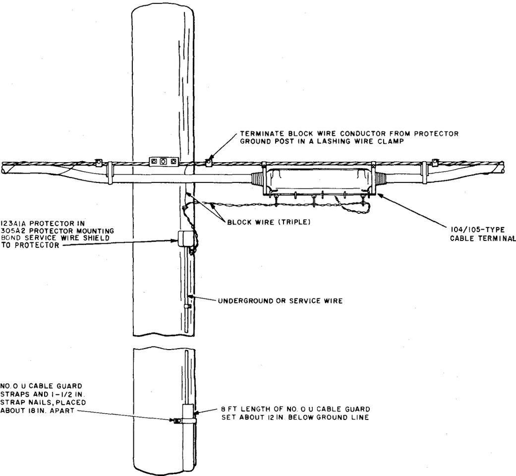
Fig. 28—Termination for Special Lightning Protection
