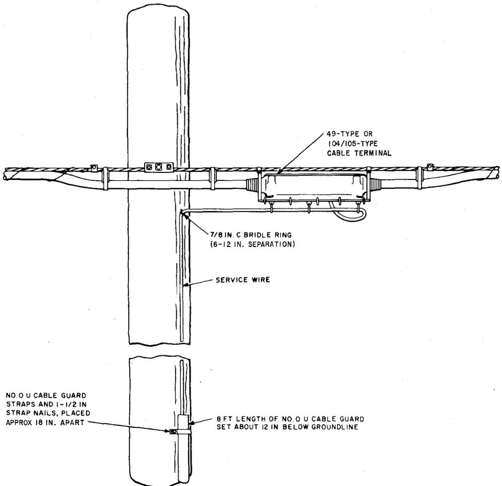
**Fig. 25—Buried Plant Run Up a Pole**
