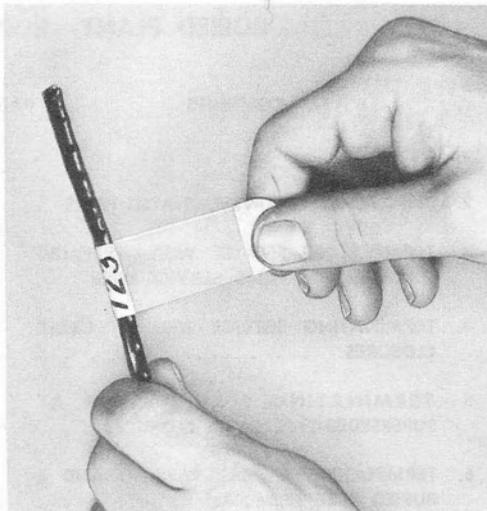
Fig. 1—♦Placing Self-Laminating Label♦
