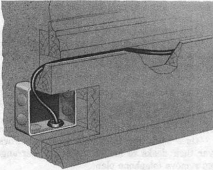
**Fig. 5—Wiring From Conduit to Baseboards**
