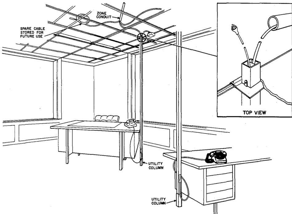
⚡ Fig. 10—Wiring Method With Utility Columns ⚡
