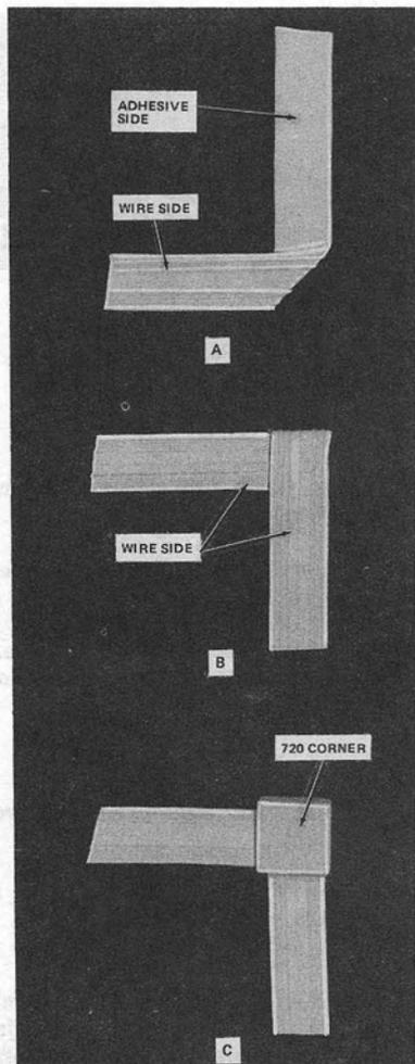
Fig. 4—90° Turn in B Station Wire
