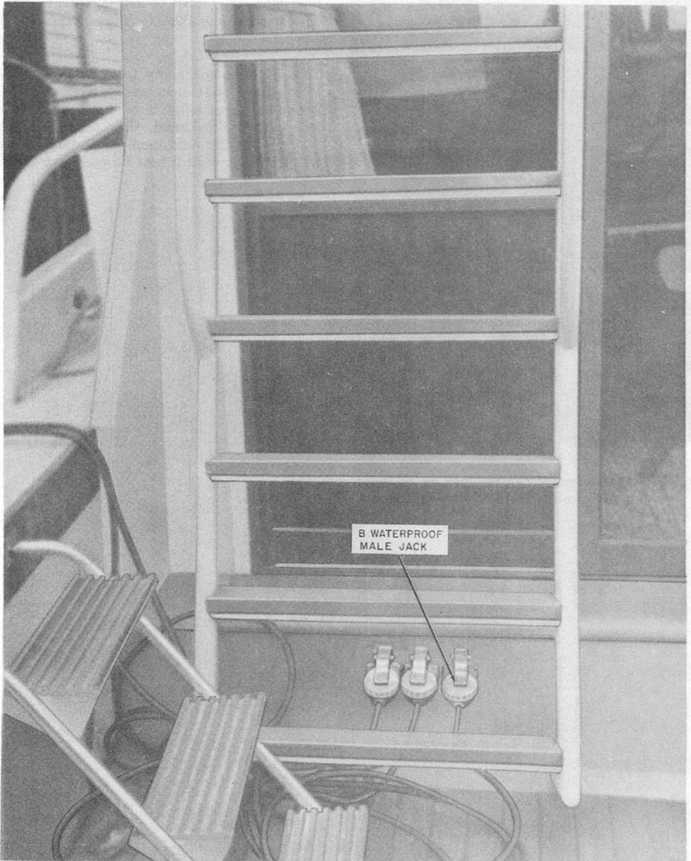
**Fig. 21—Typical Boat Coaming B Waterproof Male Jack Installation**
