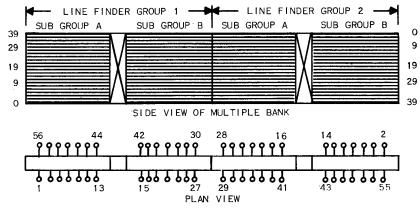
ARRANGEMENT OF MULTIPLE BANK USED FOR TERMINATING 800 LINES PER FRAME 400 LINES MULTIPLED BEFORE A MAXIMUN OF 28 LINE FINDERS
