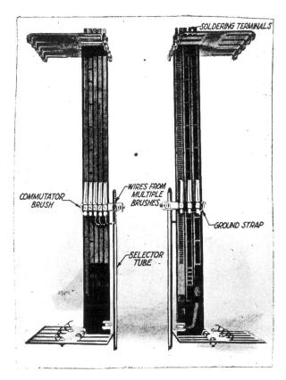
Figure 5-5 Panel Commutator Mechanism
