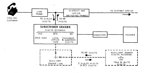
Figure 5-14 Block diagram of auxiliary sender applied to a panel central office.
