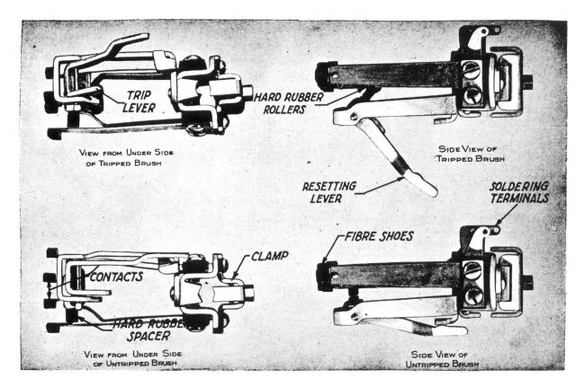
Figure 5-6 Panel Brush Mechanism
