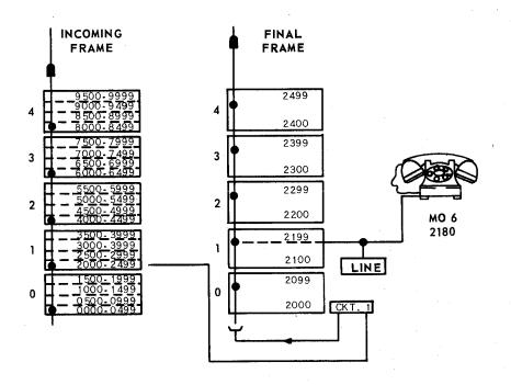
Figure 5-13 Trunking Between Incoming and Final Frames
