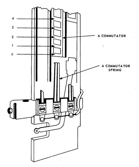
Figure 5-16 "A" Commutator Segments
