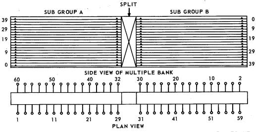
ARRANGEMENT OF MULTIPLE BANK USED FOR TERMINATING 400 LINES PER FRAME 400 LINES MULTIPLED BEFORE A MAXIMUM OF 60 LINE FINDERS
