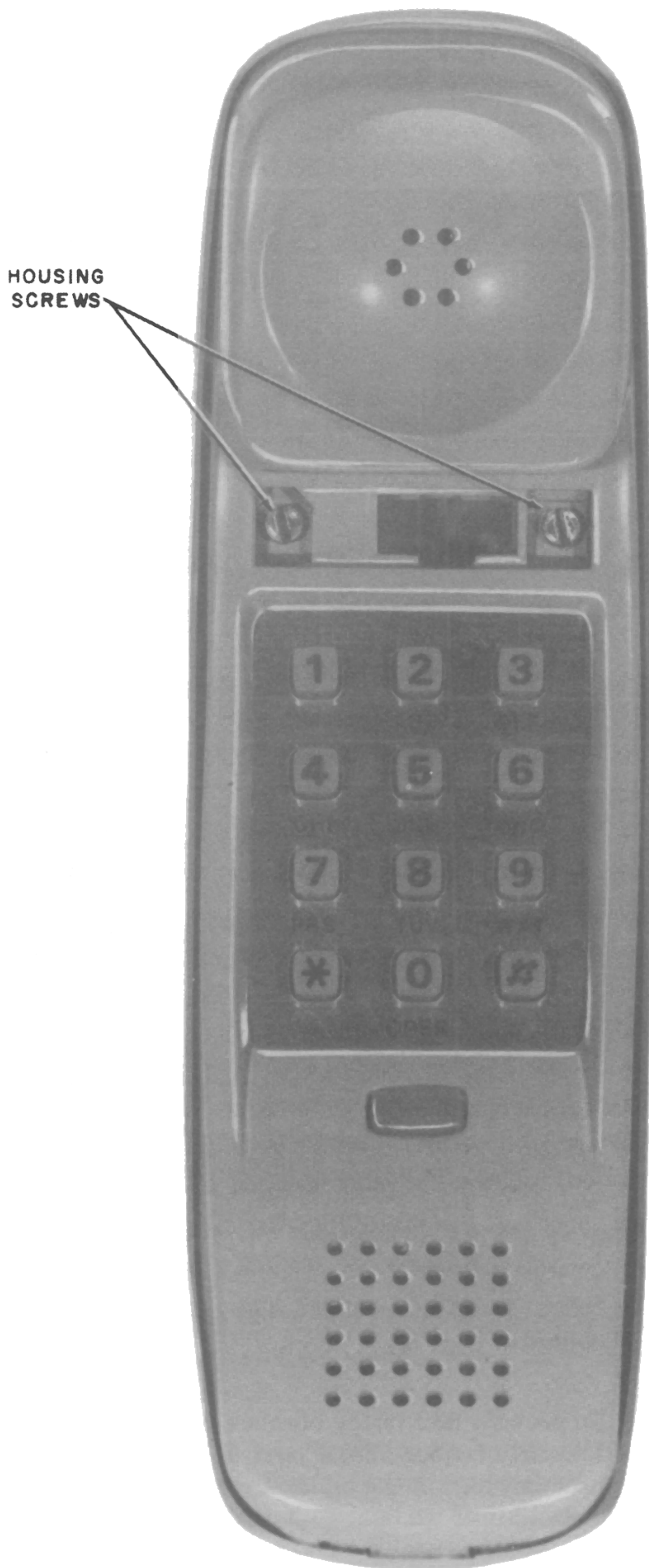
Fig. 6—Location of Housing Screws
