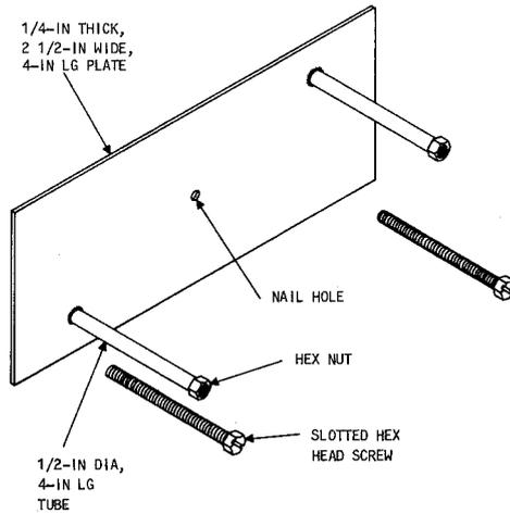
Fig. 8—Twin-Bolt Fastener
