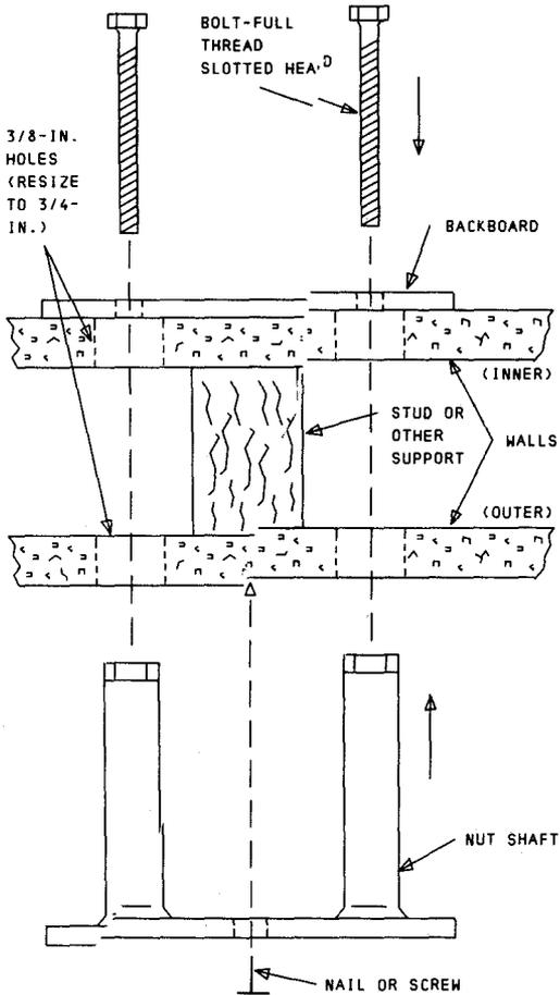
Fig. 10—Twin Bolt Fastener Installation
