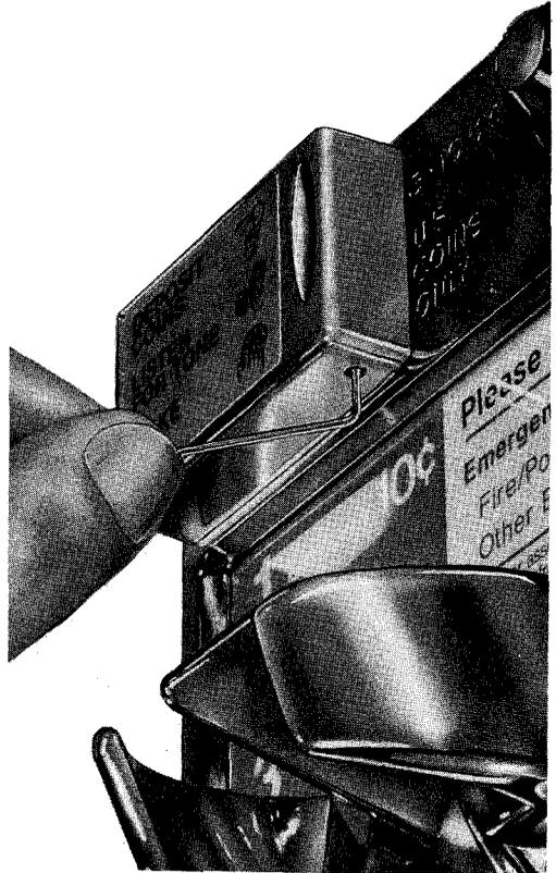
**Fig. 57—Setscrew Adjustment**
