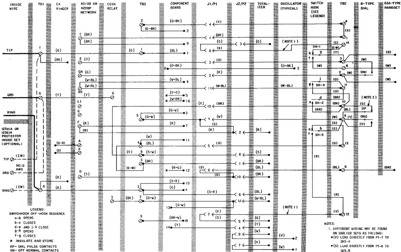
Fig. 67—1C1 or 2C1 Coin Telephone Set—CF Connections
