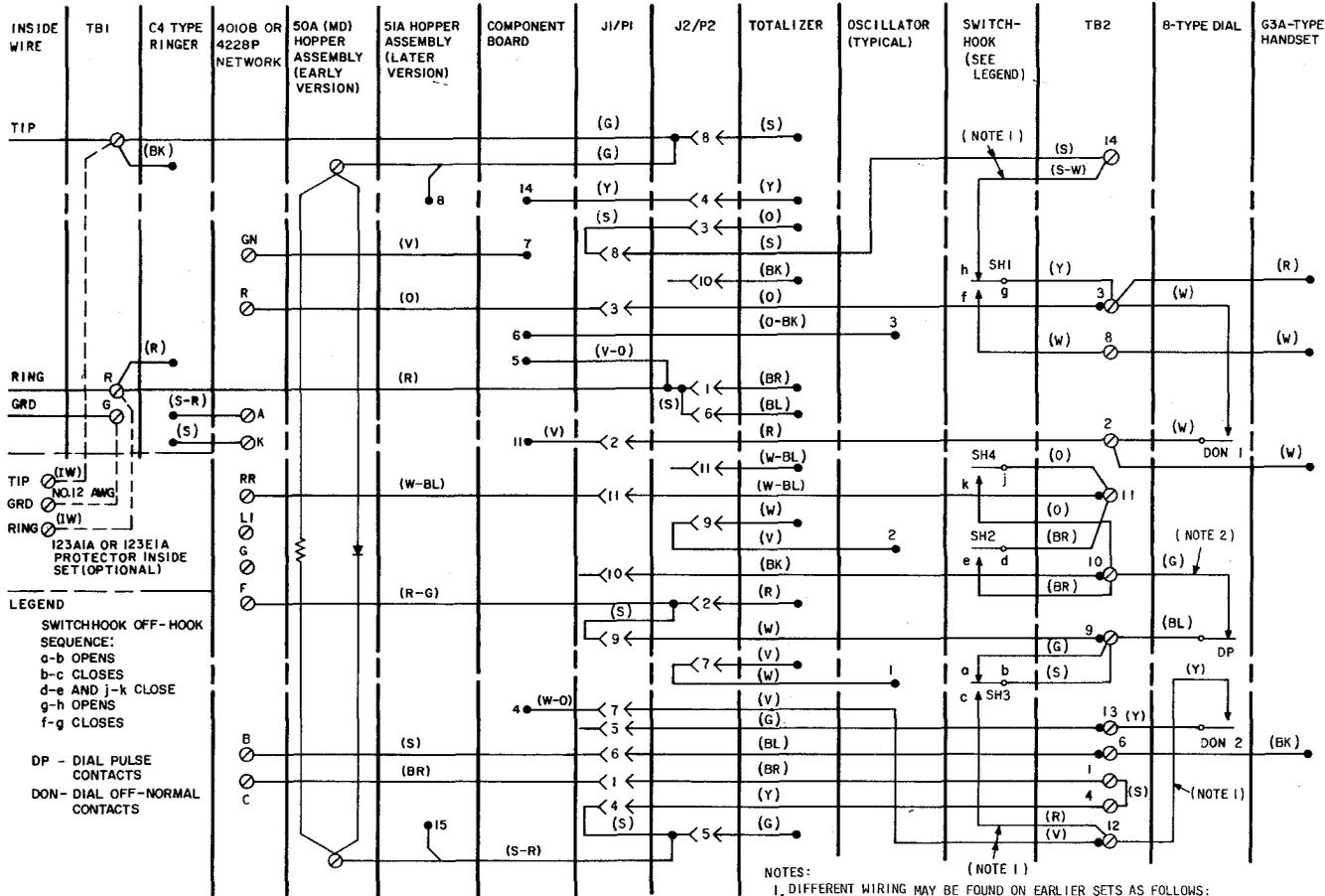
Fig. 73—1E1 Coin Telephone Set—Connections
