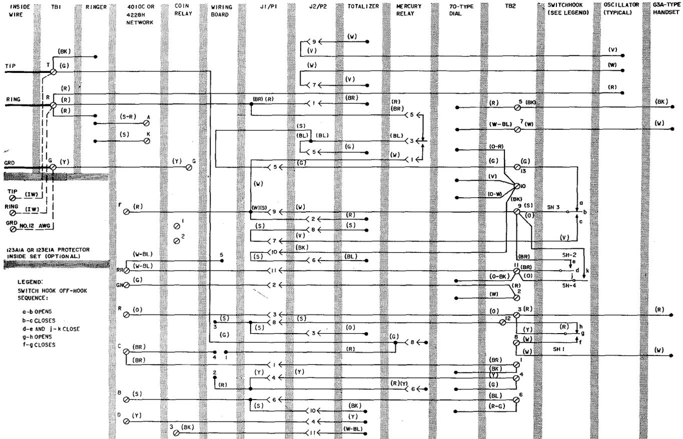
Fig. 66—1A2 or 2A2 Coin Telephone Set W/70-Type Dial—Connections
