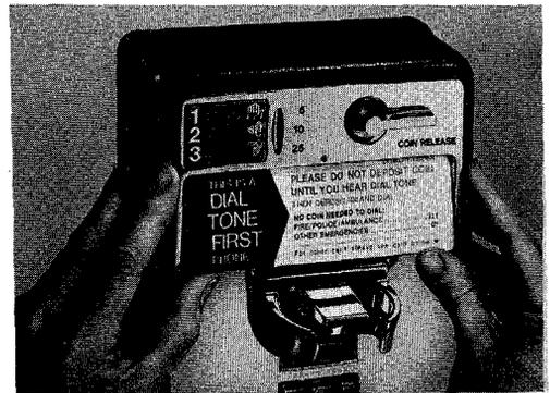
**Fig. 20—Installing Instruction Cards in 1-Type Set (Typical)**
