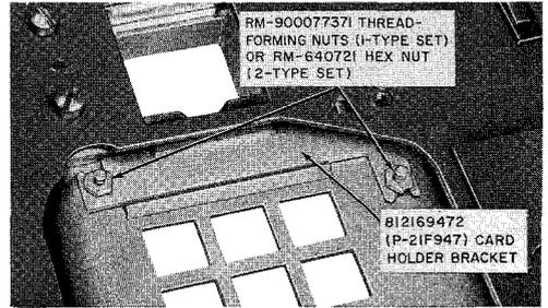
**Fig. 29—Card Holder Bracket Installed in TOUCH-TONE Set**
