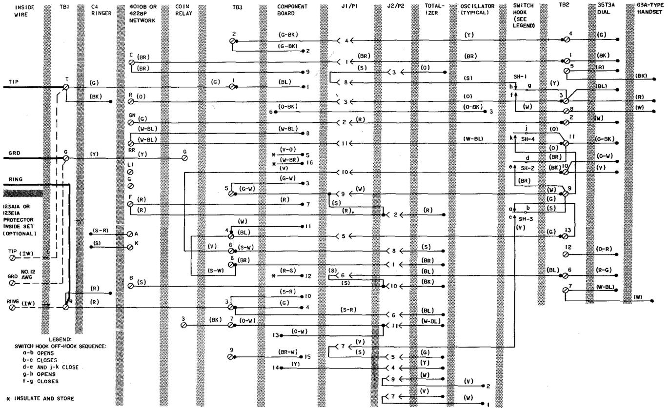
Fig. 69—1C2 or 2C2 Coin Telephone Set W/35T3A Dial—CF Connections
