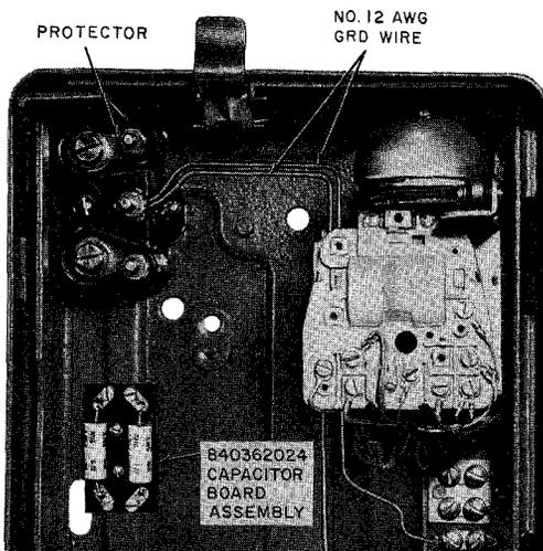
**Fig. 51—Housing and Mounting Plate Assembly**
