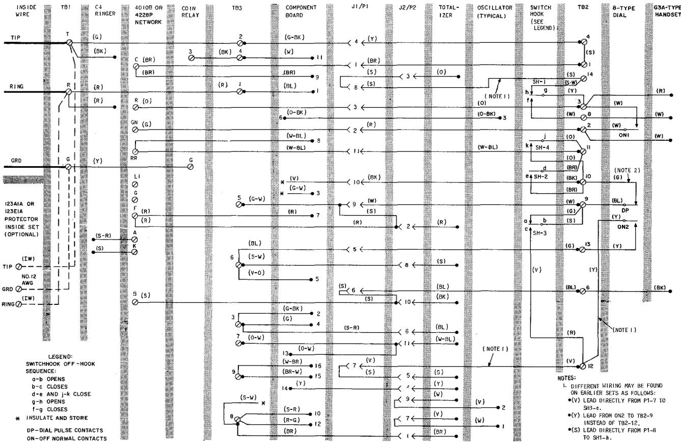
Fig. 68—1C1 or 2C1 Coin Telephone Set—DTF Connections
