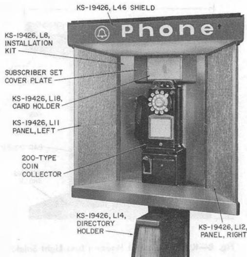
**Fig. 11—KS-19426 Mounting Using 200-Type Coin Collector**
