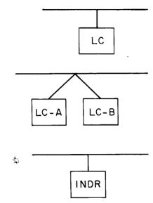
**Note:** Along with each load coil or inductor case symbol or combination thereof, the load point identification, location, number and type of coils or inductors, cable count and any other information so dictated by Operating Company policy or forthcoming Bell System Practices must be shown on both work prints and records.
