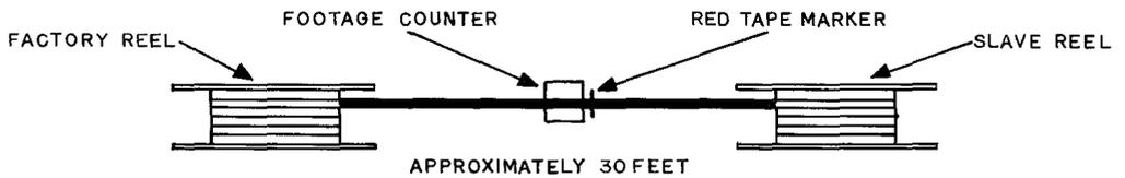
Fig. 11—Placing Short Section on Slave Reel
