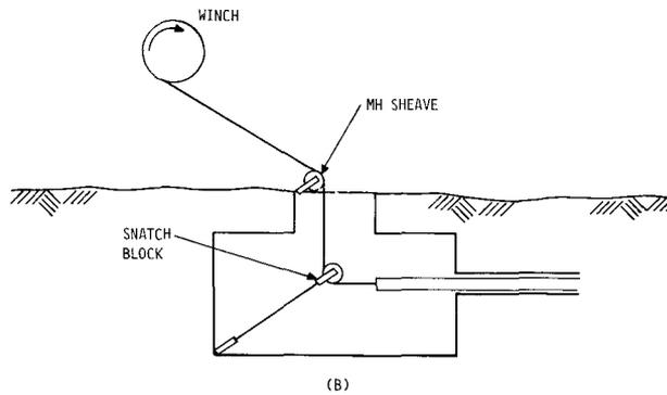
**Fig. 9—Innerduct Sweep vs Blocks at the Pull Manhole**
