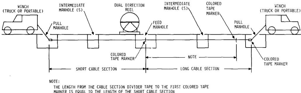
Fig. 12—Location of Cable Tape Markers
