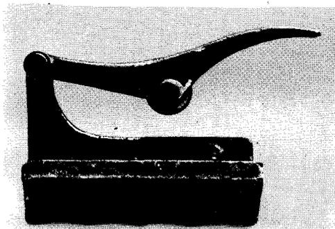
**Fig. 1—Innerduct Slitter (AT-8959)**
