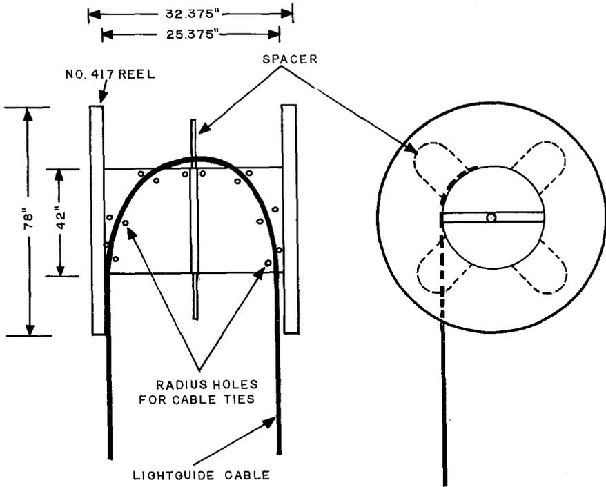
Fig. 10—Typical Reel Modification
