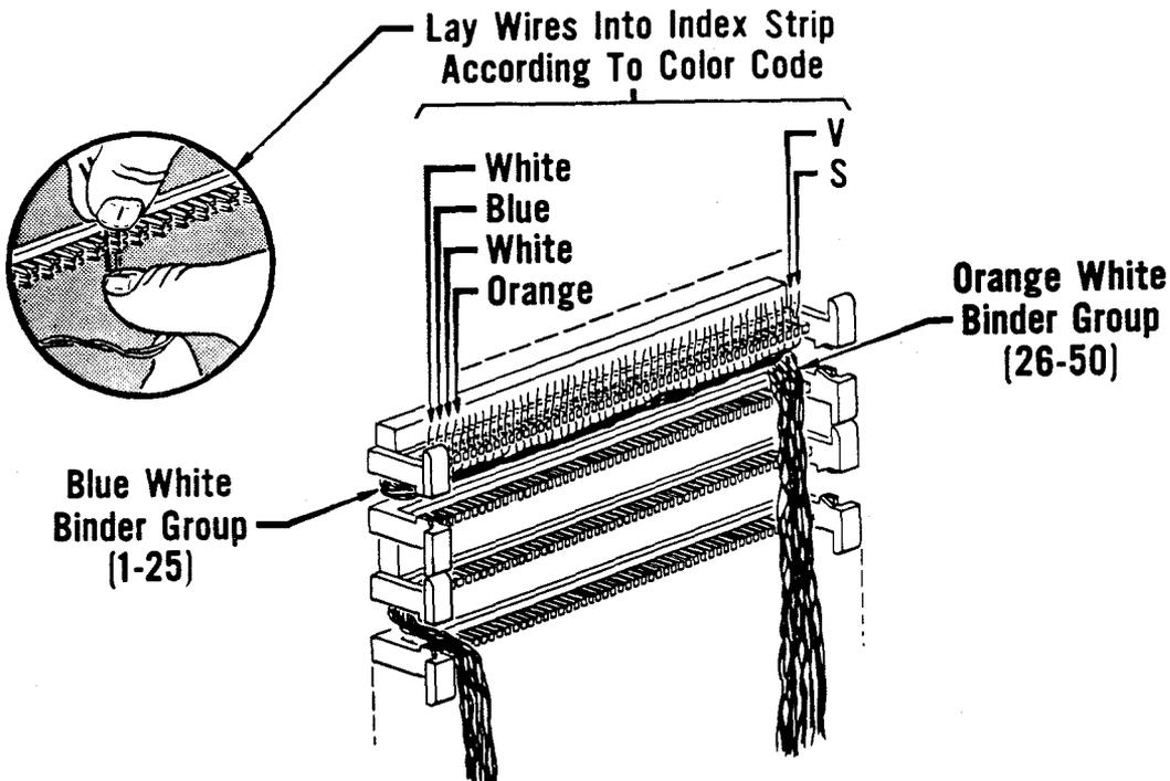
**Step 19—Placing Conductors Into Index Strip**
