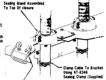
Step 7—Installation of Bond Assemblies and Sealing Gland for Top Entrance Cables
