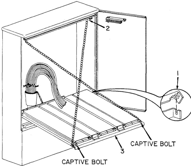
**Step 4—Installation of Mounting Frame**
