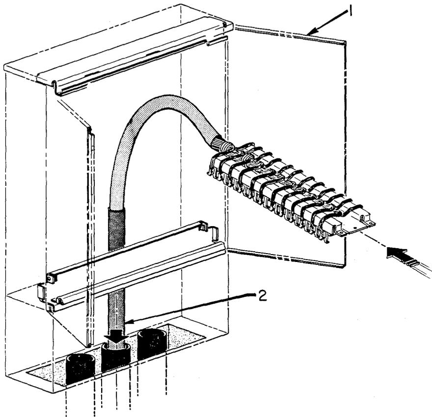
**Step 9—Installing Terminal Block in Cabinet**
