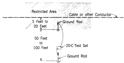
**Fig. 7—Two Ground Rod Connection**
