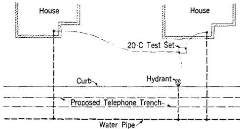
**Fig. 4—Direct Connection At Two Points—Conductors of Other Utilities**
