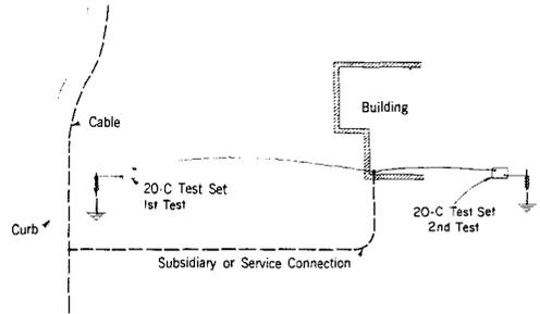
**Fig. 6—One Direct Set and One Ground Rod**
