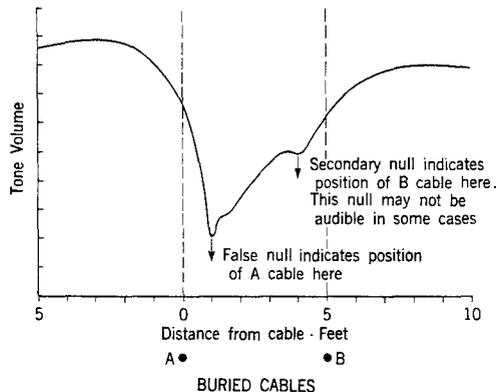
**Fig. 12—Two Conductors on Same Route**
