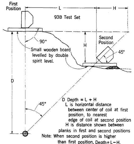
**Fig. 11—Depth Measurements over Ground That is Not Level**
