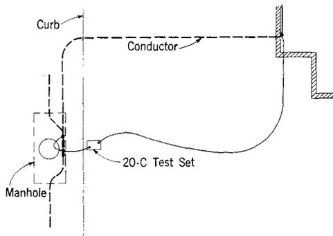
**Fig. 5—Direct Connection At Two Points—Buried Subsidiary Cable or Service Connection**
