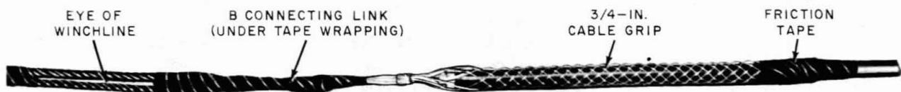
Fig. 14 — Cable Grip and Winch Line Attached
