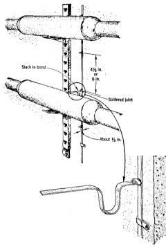
2.04 If the permanent bond is installed without projections the piece of bonding ribbon to the sleeve of the cable is attached to the permanent bond as shown below.
