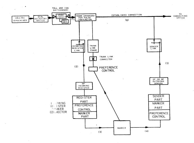
Figure 8-20 Pulse Conversion Operation
