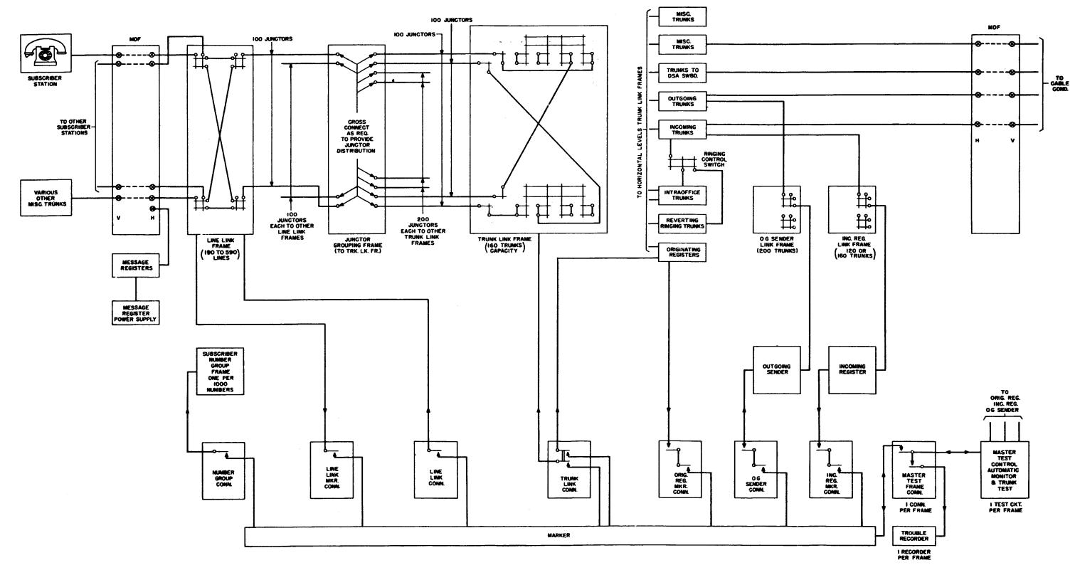
Fig. 8-1 - Equipment Schematic of No. 5 Crossbar Office
