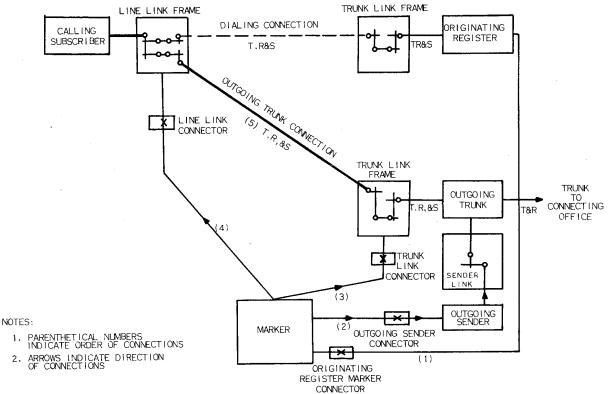
Figure 8-12 Outgoing Trunk Connection
