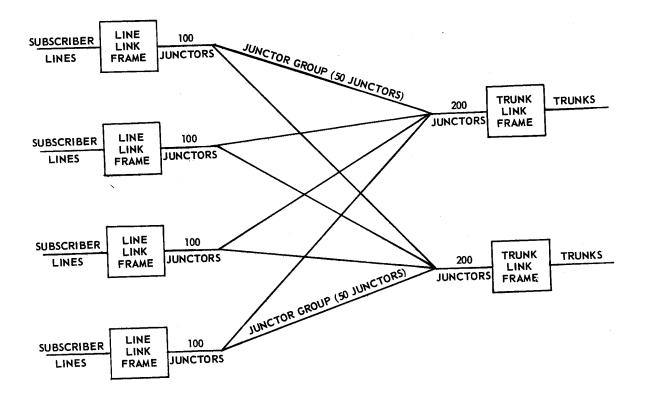
Figure 8-6 Junctor Distribution (4 Line Link and 2 Trunk Link Frame)
