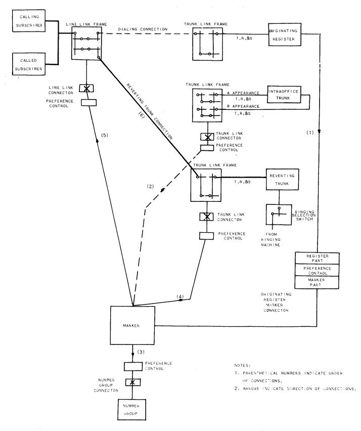
Figure 8-16 Reverting Trunk Connection
