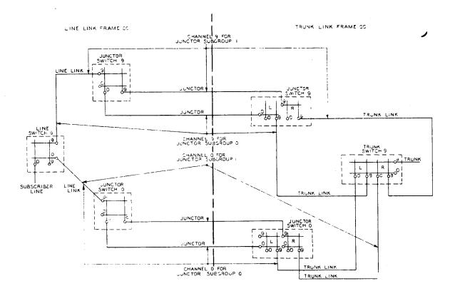
Figure 8-9 Channel Distribution -- Line Link to Trunk Link Frames
