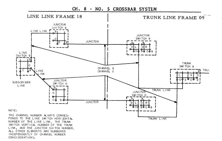
Figure 8-8 Channels for 20 Line Link-10 Trunk Link Frames
