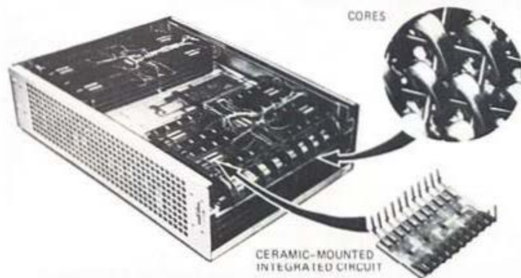
Fig. 5-6: The 20A memory module, which contained 851,968 cores with two wires threaded through each core. For increased functional density, several integrated circuits were mounted on ceramic units, which in turn were assembled on a printed circuit board. The module was organized as 32,768 words of 26 bits.
