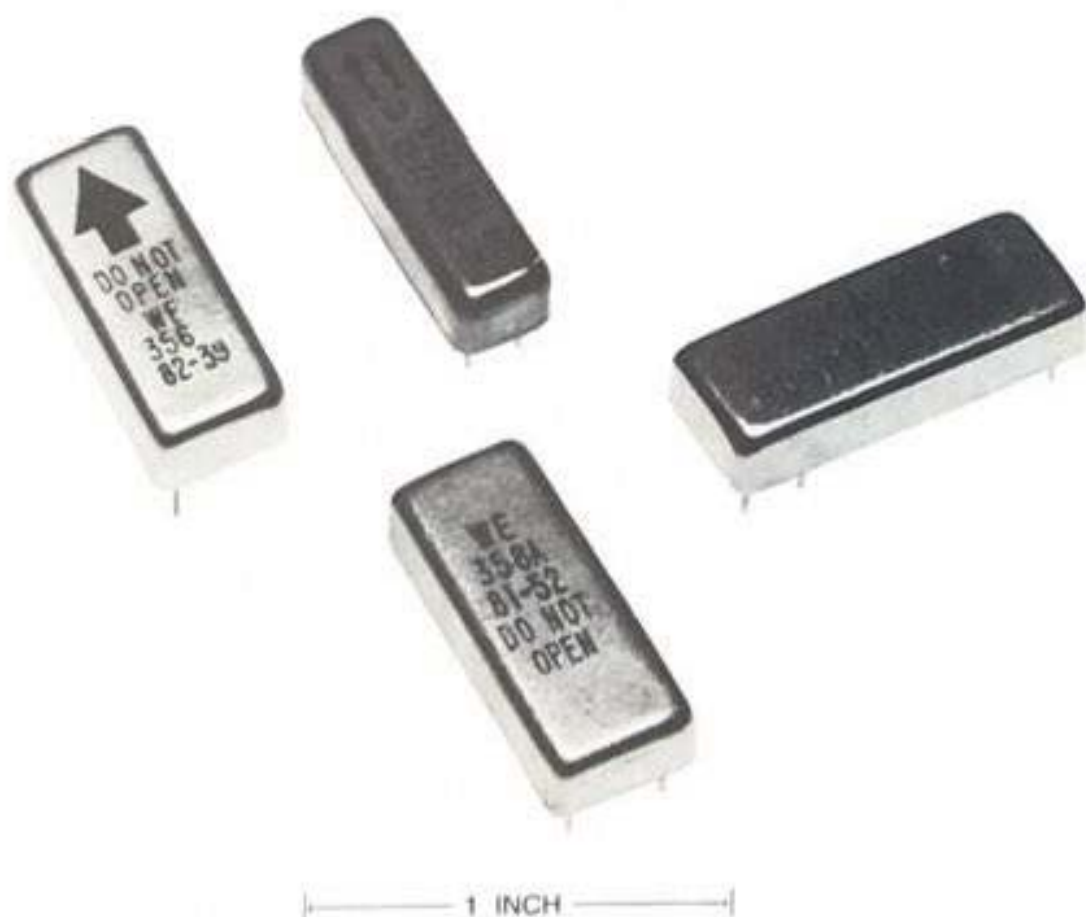
Fig. 7-11. Examples of the miniature mercury relay family. The 345-type and 356-type relays (marked with arrows) require fixed mounting orientation. The 354-type and 358-type relays can be mounted in any position.
