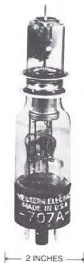
Fig. 3-12. The 707A, the first reflex klystron designed for voltages as low as 300 V, an advantage for radar equipment.
