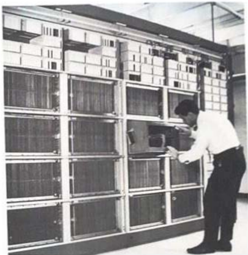
Fig. 5-13. Program store of the Succasunna, New Jersey electronic switching system office. More than 5 million bits of information were stored in 16 modules of permanent-magnet twistor memory.
