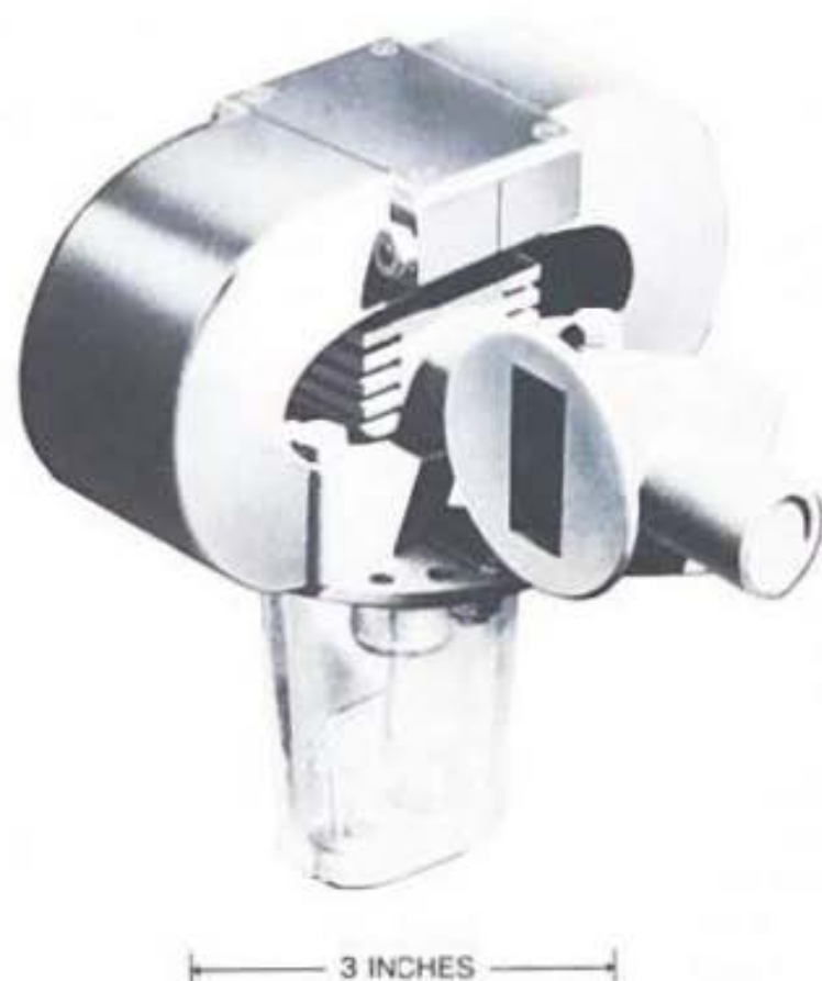
Fig. 3-19. The 2J55 packaged tube magnetron, which featured an external magnet as an integral part of the device. Magnet weight and size were reduced considerably in this design.
