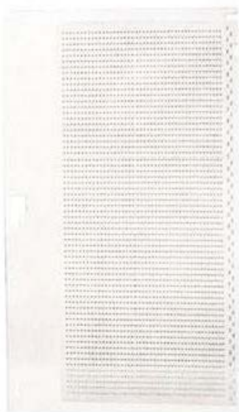
Fig. 5-12. The aluminum magnet card, which carried an array of 2816 information bar magnets and a double stripe of initializing magnets. A twistor store consisted of 16 modules of 128 cards each; an electronic switching system central office contained two to six stores.
