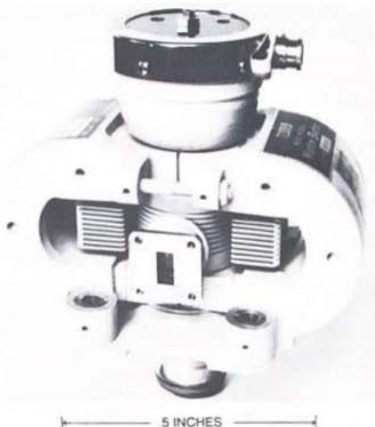
Fig. 3-20. The 7208 coaxial cavity magnetron, employed in military applications for over 30 years. Motion of a single plunger tunes the device.
