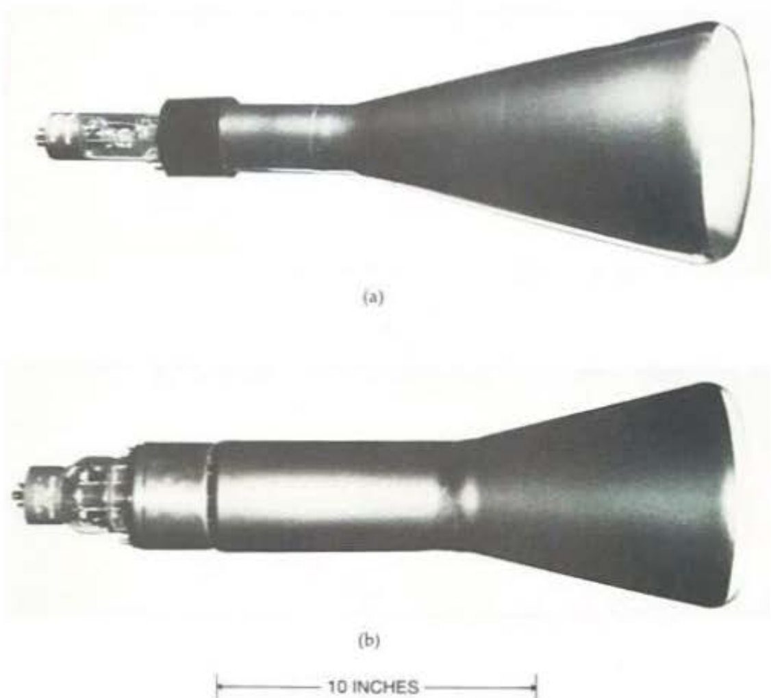
Fig. 3-8. Two Western Electric cathode ray tubes of the 1930s: (a) the 326A, which used electrostatic focusing; (b) the 330A, which had three electron guns.
