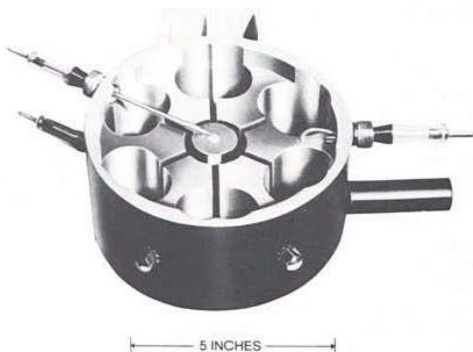
Fig. 3-17. Basic structure of magnetron oscillator for centimeter wavelength RF generation. A series of resonators with radial slots surrounds a central cylindrical cathode.
