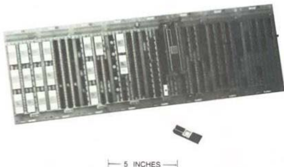
Fig. 2-13. Photo of a WE 8000 microprocessor in 40-pin package. The accompanying breadboard of SSI and MSI simulated one-half the functional complexity of the WE 8000 processor.
