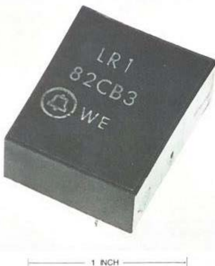
Fig. 7-6. A typical LR-type relay intended for printed wiring board mounting in solid-state systems.
