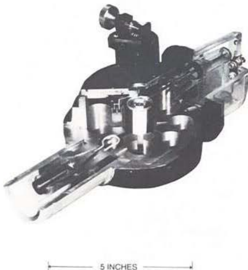
Fig. 3-18. The 4J51 magnetron, which had a vacuum diaphragm to attain smoothly controllable movement inside an envelope of resonator pins, allowing tunable frequency.
