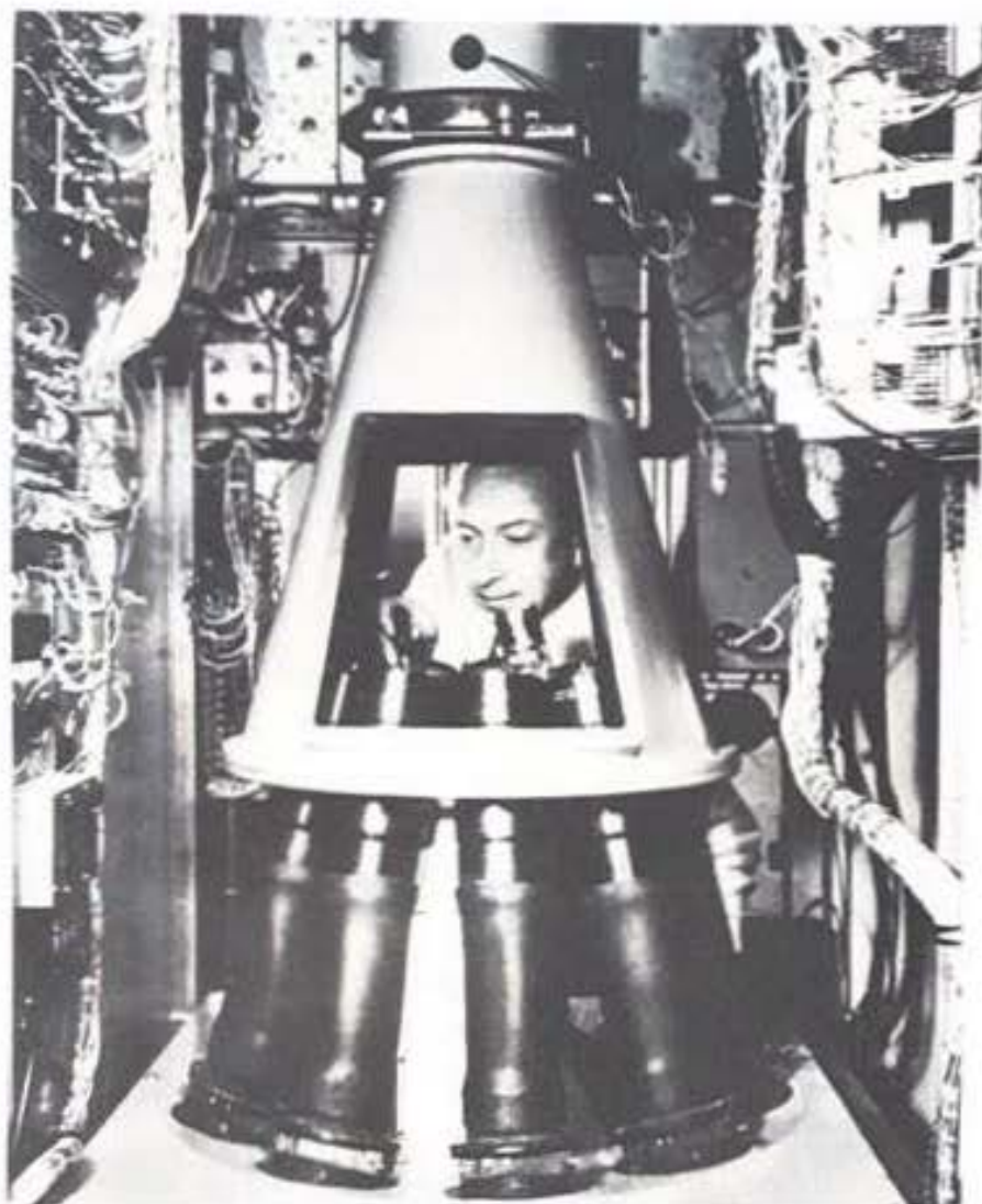
Fig. 3-42. Laboratory model of the flying spot store. Design objectives included minimum beam distortion, a phosphor screen with very fast decay, and a nearly optically perfect tube face.
