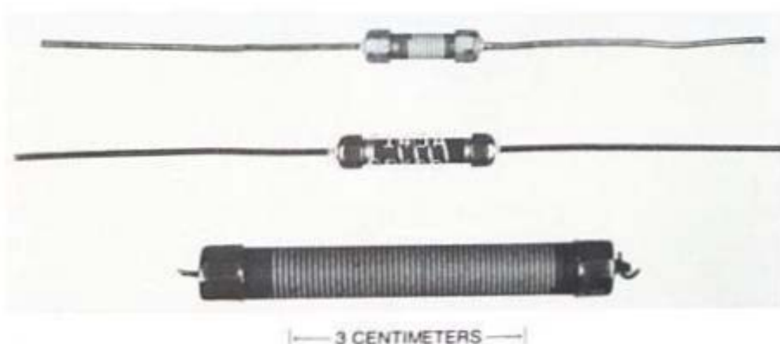
Fig. 8-10. Carbon film resistors, made by grinding helical grooves through the film by automated machinery developed by Western Electric engineers.
