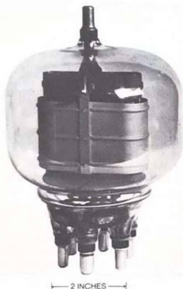
Fig. 3-23. The 363A pentode, used in ultrahigh-frequency radio telephony transmission across the Chesapeake Bay in 1941. It operated most efficiently between 30 and 85 MHz.
