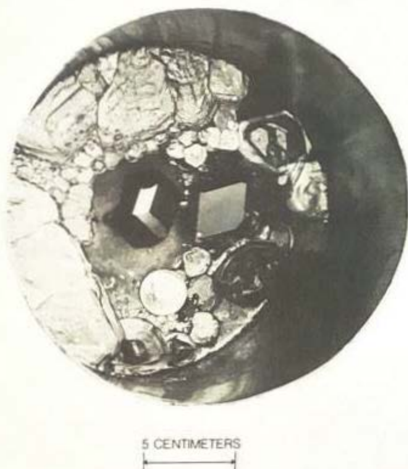
Fig. 5-18. Platinum crucible containing dozens of garnet crystals grown from a molten flux solution by L. G. Van Uitert. Many of the larger crystals were sliced and polished for device evaluation.
