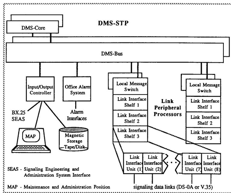
Figure 5. DMS-STP Architecture
