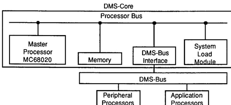
Figure 2. DMS-Core Architecture
