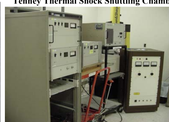
In-House Hi-Power Testing (TWT's up to 200-Watts)
