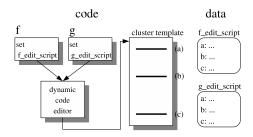
Fig. 1. Run-time code mutation with clustered procedures
