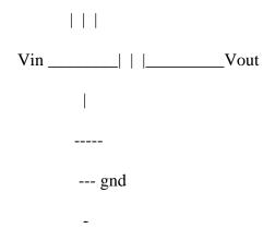
Vin = Voltage in, 6-12 volt wall adaptor, + goes to Vin, - goes to gnd
