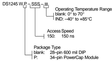
**DS1245W NONVOLATILE SRAM, 32-PIN 740 MIL EXTENDED DIP MODULE**
