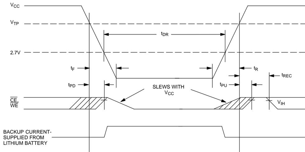
**POWER-DOWN/POWER-UP TIMING**(t<sub>A</sub>: See Note 10)
