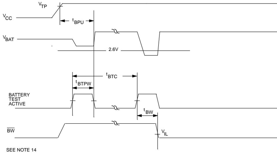
**POWER-DOWN/POWER-UP TIMING**(t<sub>A</sub>: See Note 10)
