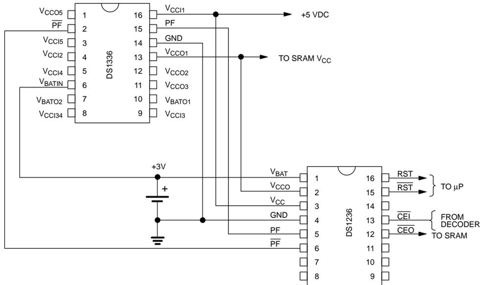
**DALLAS SEMICONDUCTOR DEVICES WHICH PROVIDE PF OR  $\overline{\text{PF}}$  INPUT TO NIL** Table 1
