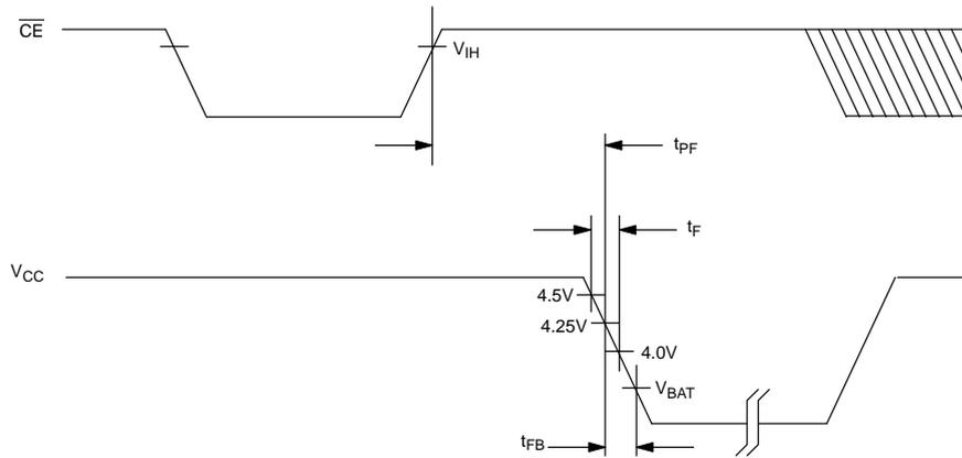
**AC ELECTRICAL CHARACTERISTICS POWER-UP POWER-DOWN TIMING** (0°C to 70°C)
