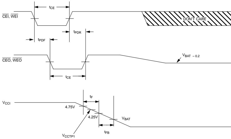
**TIMING DIAGRAM: POWER UP (3 VOLT)**
