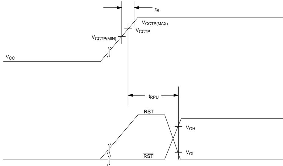
**$\overline{RST}$  VALID TO 0 VOLTS  $V_{CC}$**  Figure 8
