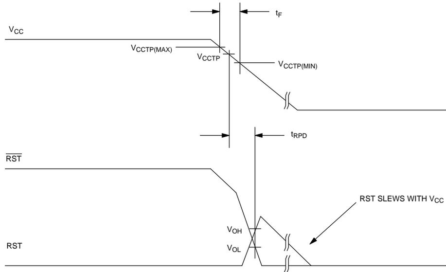
**TIMING DIAGRAM: POWER UP** Figure 7
