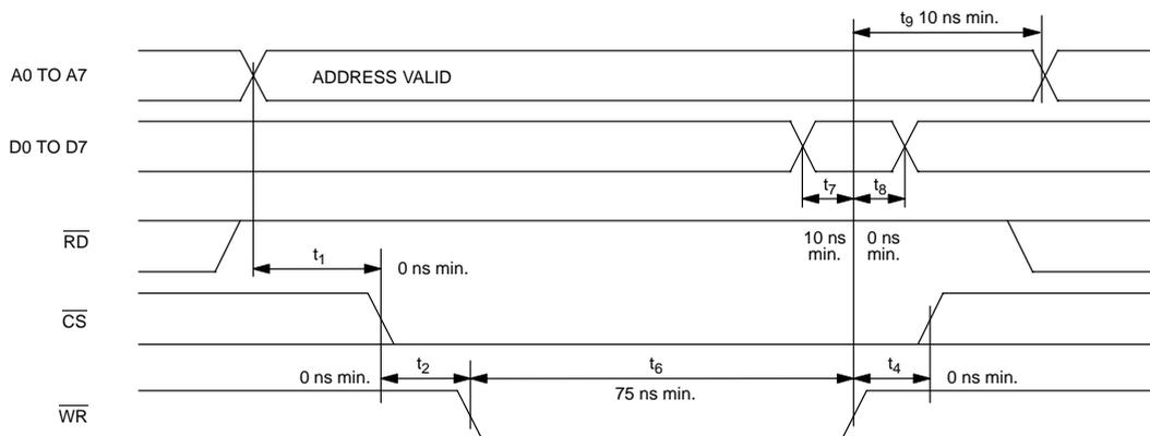
**MOTOROLA BUS READ AC TIMING (BTS=1/MUX=0) Figure 16-12**
