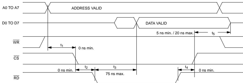
**INTEL BUS WRITE AC TIMING (BTS=0/MUX=0) Figure 16-11**
