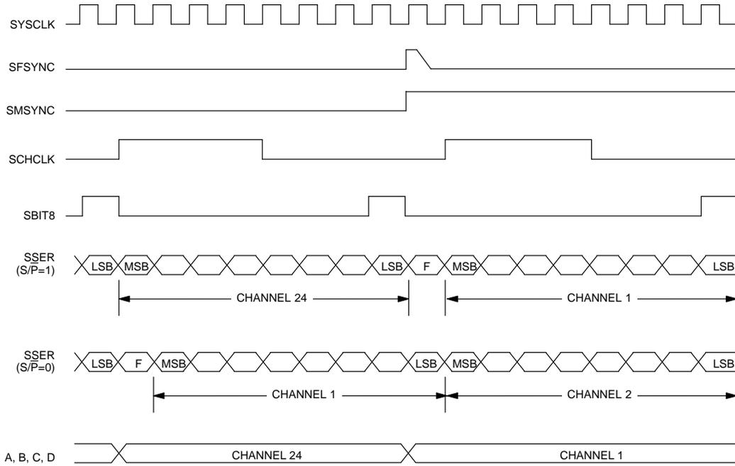
**SYSTEM MULTIFRAME BOUNDARY TIMING (SYSCLK = 2.048 MHz) Figure 4**
