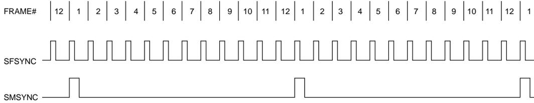
**193E SYSTEM MULTIFRAME TIMING** Figure 6
