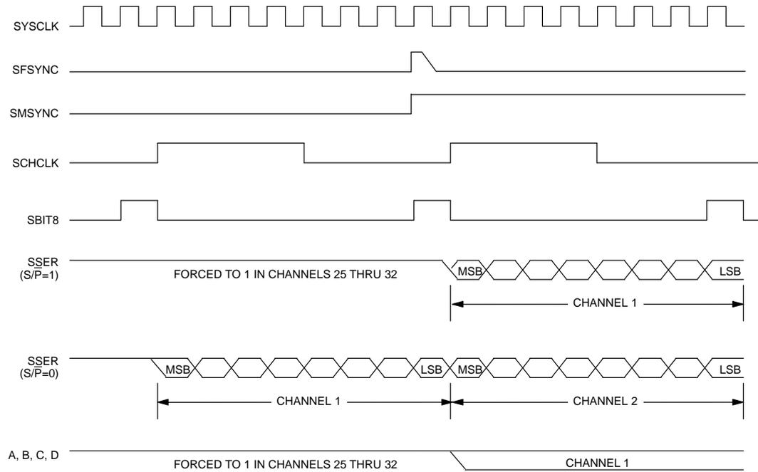
**193S SYSTEM MULTIFRAME TIMING** Figure 5
