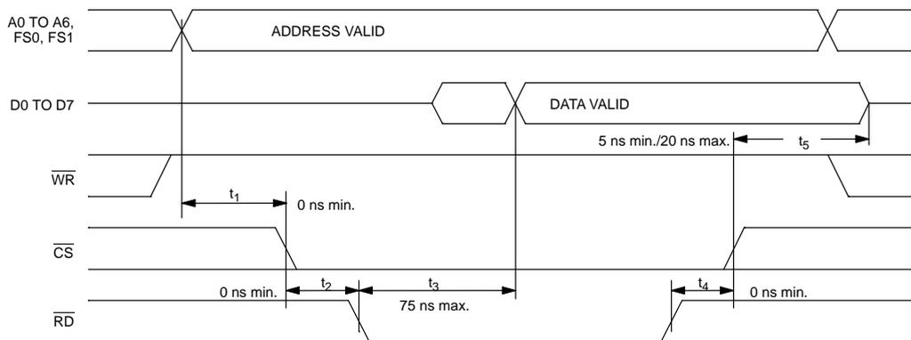
**INTEL BUS WRITE AC TIMING (BTS=0/MUX=0) Figure 13-11**
