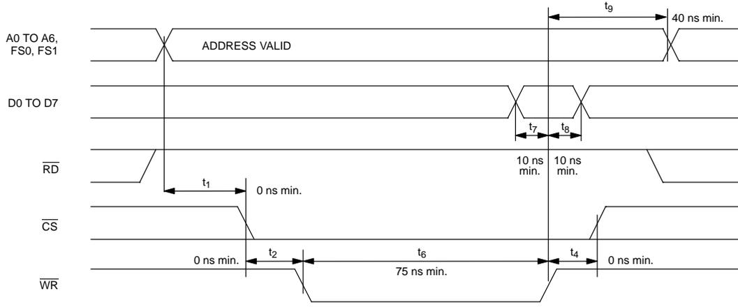
**MOTOROLA BUS READ AC TIMING (BTS=1/MUX=0) Figure 13-12**
