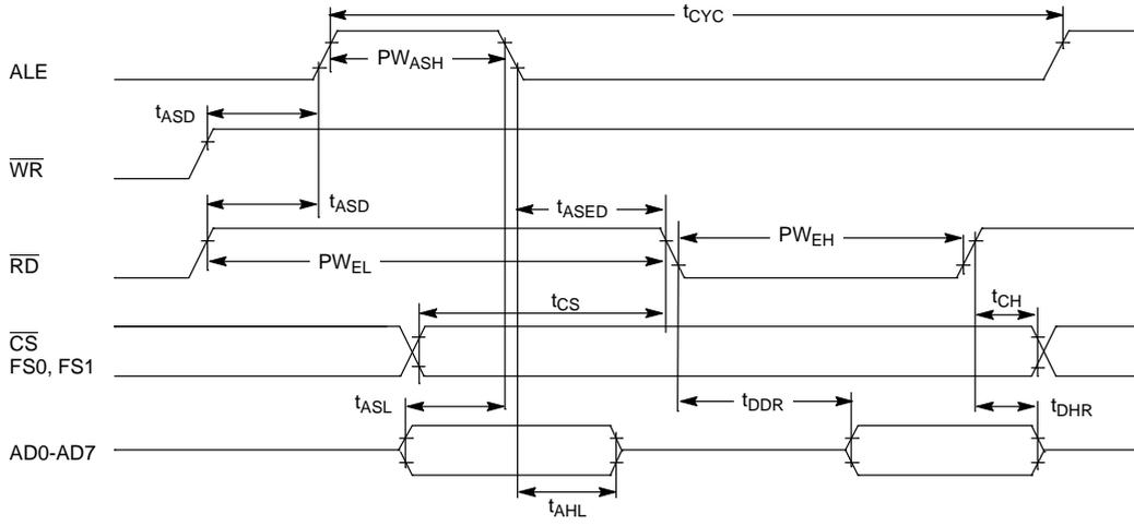
**INTEL BUS WRITE AC TIMING (BTS=0/MUX=1) Figure 13-2**
