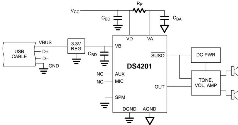
**DUAL SUPPLY CONFIGURATION, SPM=1** Figure 4b
