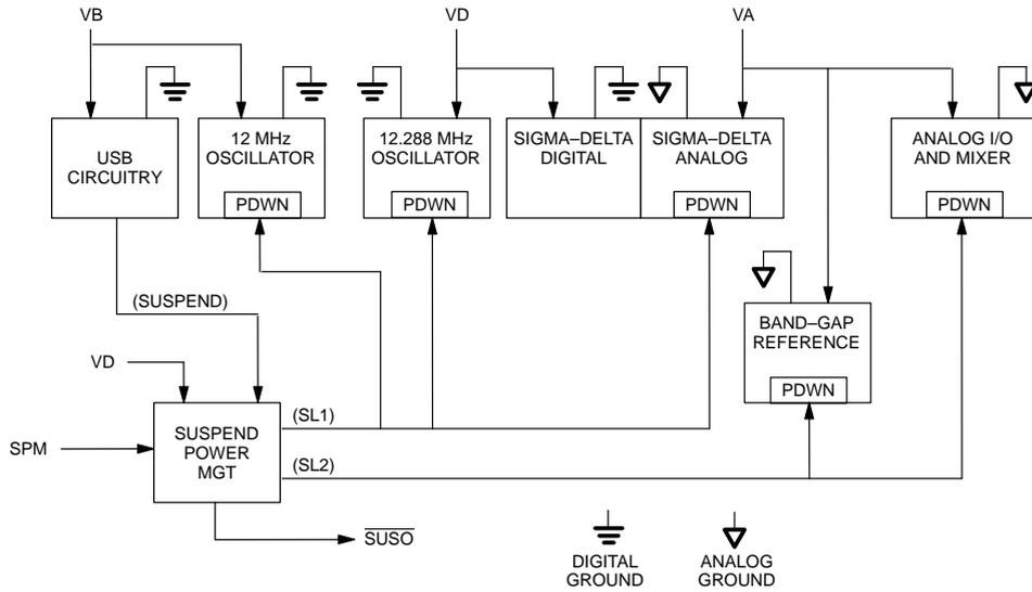
Power management in the DS4201 is controlled by the state of USB and the SPM (suspend power mode) input signal. The DS4201 was designed with the assumption that while the USB connection is active the device should be fully powered and ready to accept/convert digital audio data and during USB suspend conditions the device should provide capabilities to reduce internal and external circuit power consumption. As shown in
