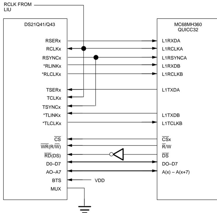
\*HDLC on the FDL can be implemented either by TDM CHANNEL B or via the port by the host processor (CPU32 internal to the QUICC32).
