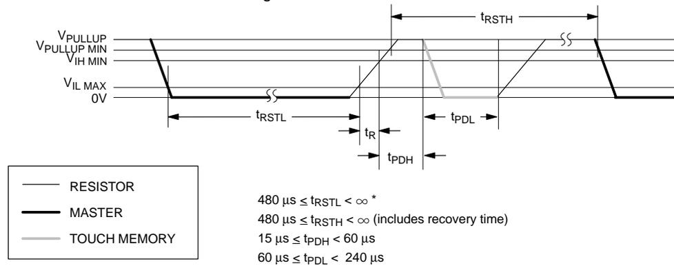
\* In order not to mask interrupt signalling by other devices on the 1-Wire bus,  $t_{RSTL} + t_R$  should always be less than 960  $\mu s$ .
