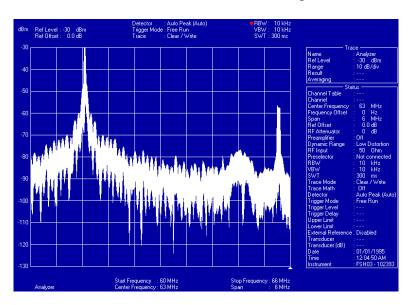
Figure 2 - This graph shows a measurement of the RF output of an NTSC signal generator, operating on TV channel 3. In this test, the modulation was set to produce a black and white raster, although the chroma carrier and aural carrier are present. These data were taken using a peak detector, with a 10 kHz bandwidth, the closest possible bandwidth to the 15 kHz bandwidth used in the test-result report.
