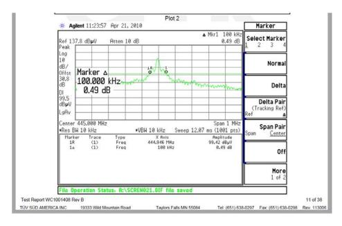
Figure 1 - This graph from the test-result report shows the measured bandwidth of the Scout when operated on with an apparent video carrier at 445 MHz.
