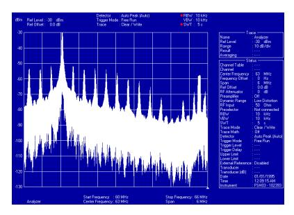
Figure 3 -- This graph shows a measurement of ARRL's NTSC signal generator, operating on TV channel 3. In this test, the modulation was set to produce a crosshatch pattern, known to be a modulation with a significant amount of black, increasing the amount of energy present in the modulation sidebands. These data were taken with a peak detector in a 10 kHz bandwidth.
