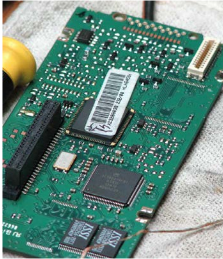
Figure 11.2 A Motorola Inc. ASTRO Digital Spectra™ vocon is shown with the host and DSP flash ROMs removed. This vocon was fortunate enough to receive a free firmware update. It was transformed from VSELP to IMBE™ through donor firmware cloned from another ASTRO Digital Spectra™ which had recently been flashed with the latest firmware builds.
