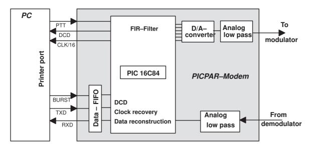
Both is realized via a burst clock generated by the PC. The PIC performes the transmitter FIR filter an the incoming data and passes the result to a 7 bit D/A converter. On the receiver branch, a lot more functions have to be carried out: First, a clock signal has to be recovered from incoming data. Then data have to be reconstructed and a carrier detection has to be performed. The regenerated data are fed into a FIFO, from where they are handed over to the PC.
