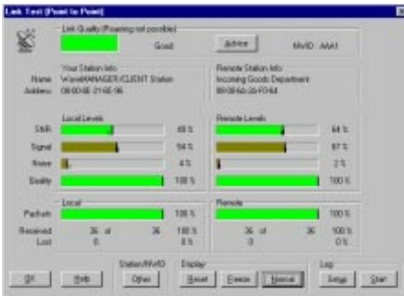
The Link Quality indicator shown in the top section of the window (in Figure 4-2) gives a first impression of the communications quality of the current link, which is the link between the local and the remote stations shown below the link quality indicator.
