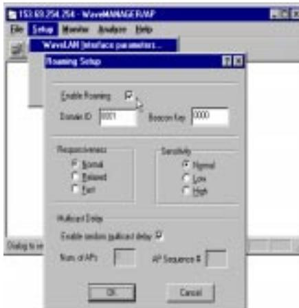
5. Click the 'Enable Roaming' check box to enable roaming.
