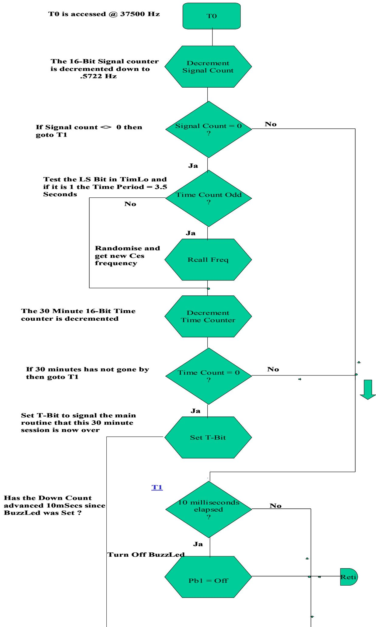
The Timer0 Overflow Interrupt Routine is called @ 37500 Hz
