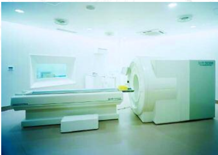
The PET camera manufactured by Hamamatsu Photonics, the SHR92000, installed at the Hamamatsu Medical Imaging Center
