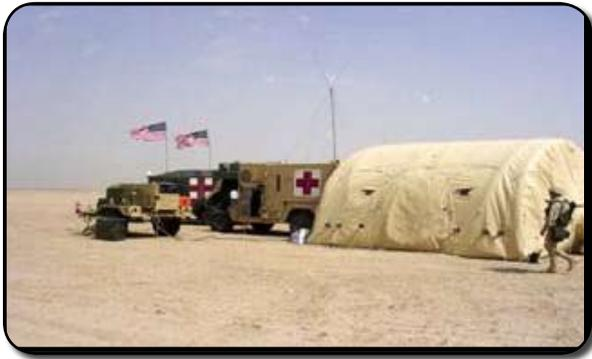
CBPS is a highly mobile, rapidly deployable shelter system designed to be used for Level I and II forward area medical treatment facilities and forward surgical teams. CBPS also replaces the M51. The CBPS consists of a dedicated M1113 Expanded Capacity Vehicle (ECV), a Lightweight Multipurpose Shelter (LMS) mounted onto the vehicle, a 300 square foot airbeam supported CB protected shelter, and a High Mobility Trailer with a towed 10kw Tactical Quiet Generator Set.
