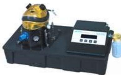
The Joint Service Mask Leakage Tester (JSMLT) is a portable test system capable of testing the serviceability of a protective mask in the field. It has expanded capability compared to the M41 PATS by allowing component level testing of the mask as well as system level testing with added components. It provides capability for an overall mask serviceability and fit factor validation of protective masks in the field.
