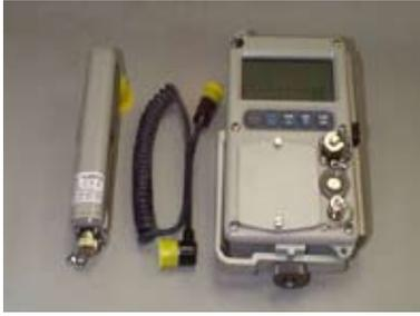
The AN/PDQ-1 RADIAC Set (MFR) consists of an IM-265/PDQ RADIAC Meter, an operator's manual, headset, carrying strap, spare batteries and the CY-8716/PDQ carrying case. The OA-9449/PDQ RADIAC Group consists of DT-680/PDQ Gamma-Beta Probe, connecting cable assembly and CY-8717/PDQ carrying case. As a stand-alone instrument, the IM-265/PDQ measures gamma radiation using an internal gamma probe. When connected to ancillary probe DT-680/PDQ it will measure beta and gamma radiation.
