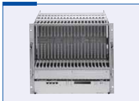
W-Ie-Ne-R VME Crate 6023 6U x 160 mm Modulformat, 9U total
