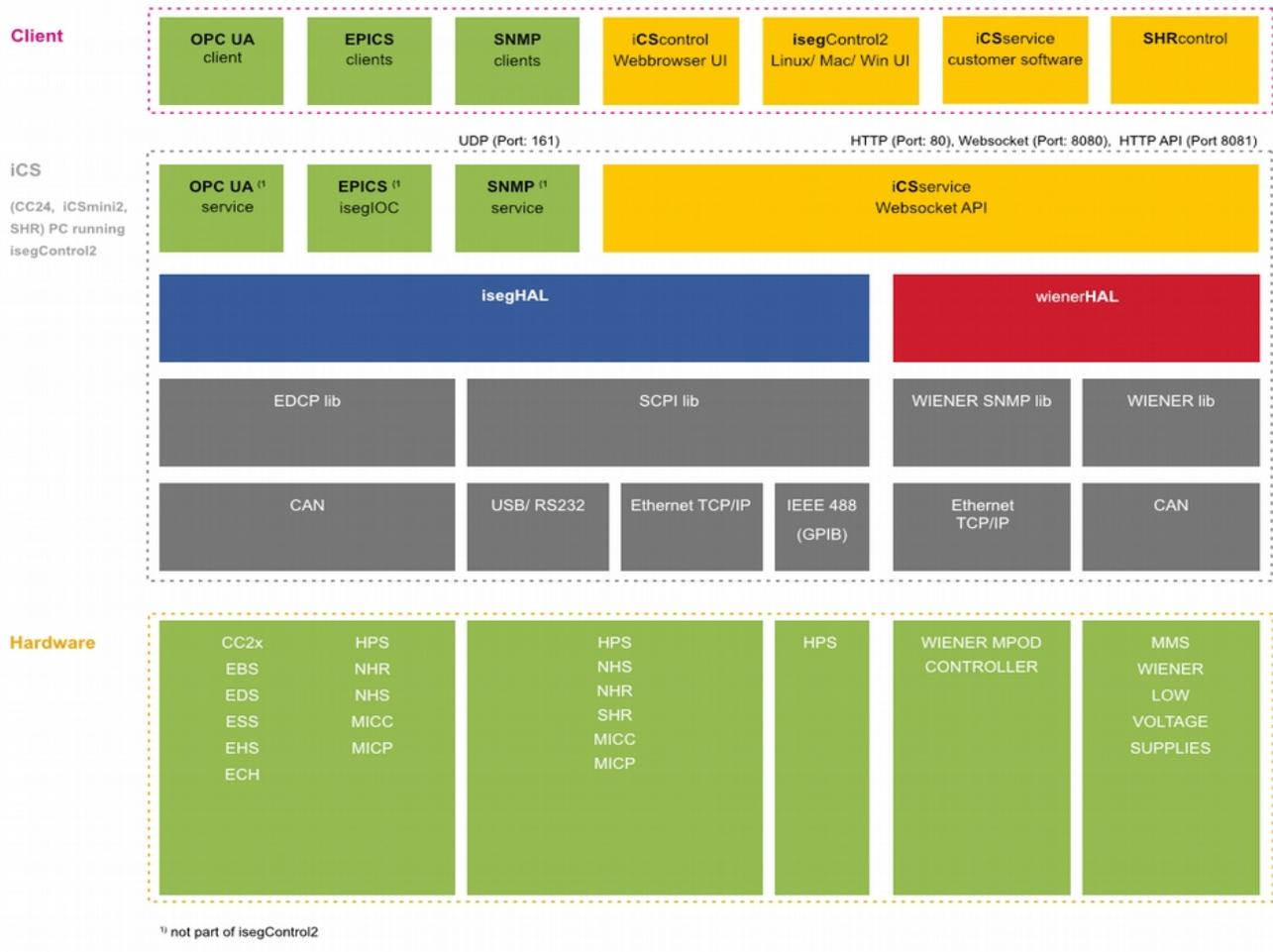
Figure 20: Software architecture
